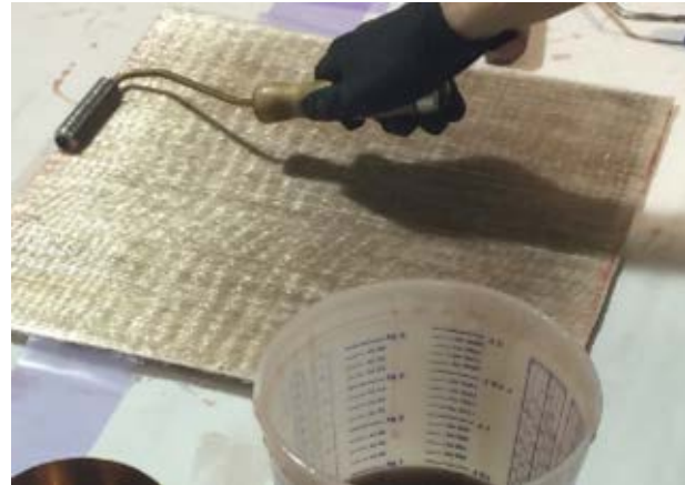
Figure 11. Metal roller for smoothing sheets
