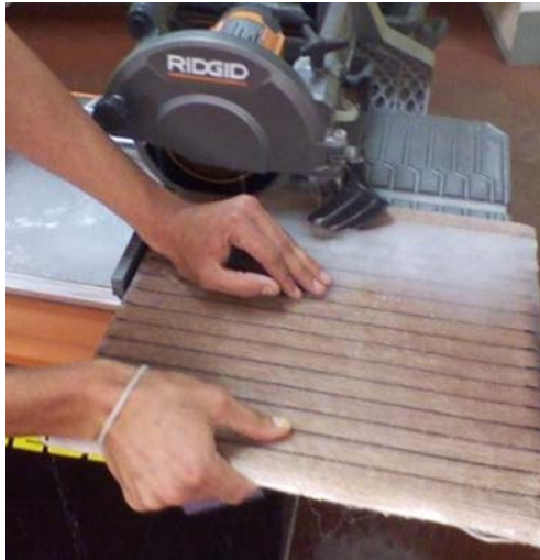
Figure 12. Cutting out specimens
