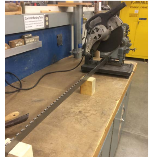
Figure 13. Cutting out hinges
