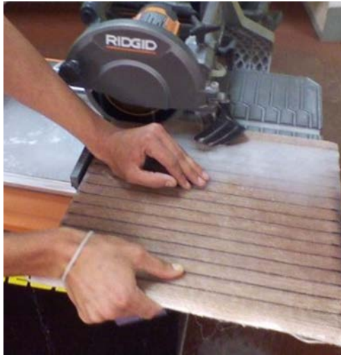
Figure 12. Cutting out specimens
