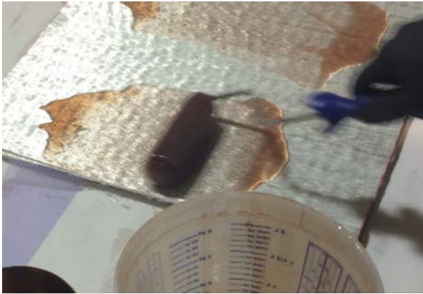
Figure 10. Foam roller for resin
