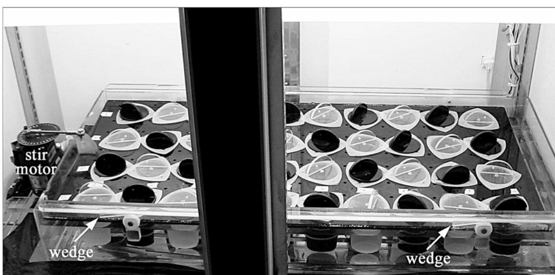
Fig. 1. Experimental tank used to maintain larvae in a homogeneous food suspension despite differences in light/dark conditions. The rollers and wedges moved the plate up and down as the stir motor moved it back and forth across the tank. This ensured mixing and exchange across the Nitex bottoms of the beakers
