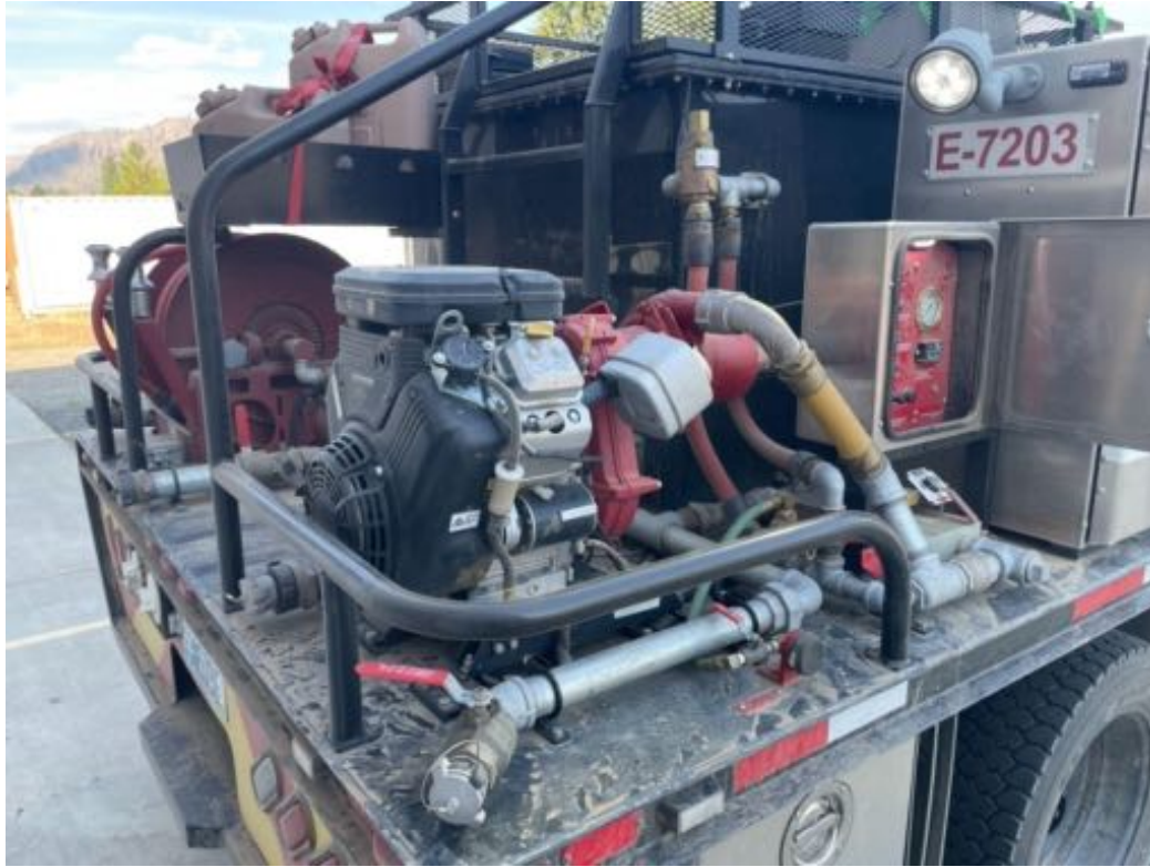
(Figure 5. The pump has multiple discharges, and can also be used for drafting water into the tank, which is when you suck water out of a nearby water body, you can even do this while actively spraying water on a fire using one
