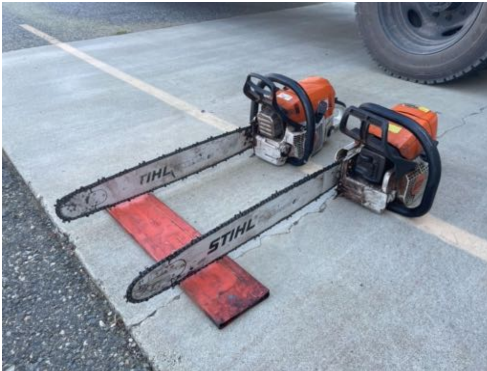
(Figure 15. The two chainsaws we kept on the truck, a Stihl 290 and 362, the 362 was to only be sharpened by the engine lead, it was also called the fire saw, because if we were on a fire we would only run the 362. The 290 could be sharpened and cleaned by crew members)
