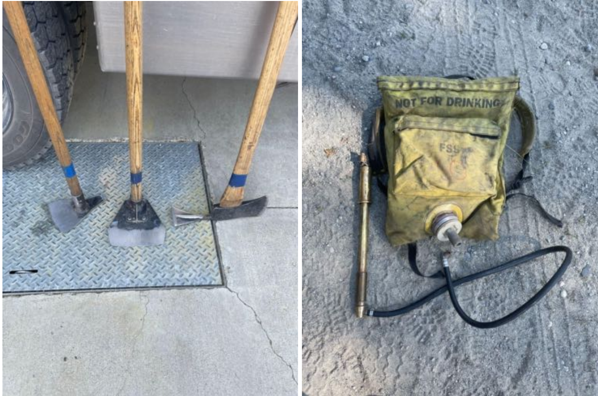
(Figure 7. Each engine has an assortment of hand tools, when crewmembers hike into a fire they generally carry a variety of hand tools to best construct the handline. Figure 8. The bladder bag is a backpack that hold 8 gallons of water, the end of the tube connects to the pack and water is sprayed out of the brass nozzle when it is pumped, they are heavy and leak)
