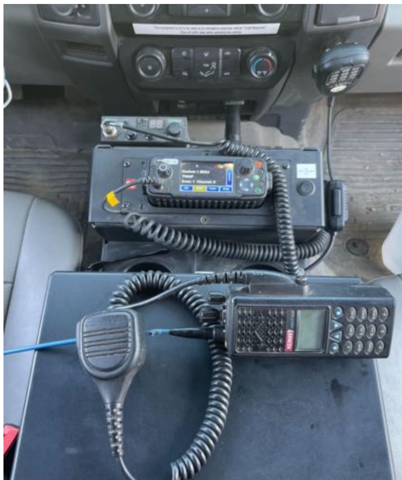
(Figure 18. It is important to learn about radio communications, we use radios constantly, to check in, in the morning and out in the evening, as well as give frequent updates on our location and status so dispatch knows what units are available and closest to incidents. Each engine gets two handheld radios, along with another in the truck, as well as a CB radio in the truck. Getting familiar with the different zones and channels is especially important when going to fires. Just remember, everyone is listening)
