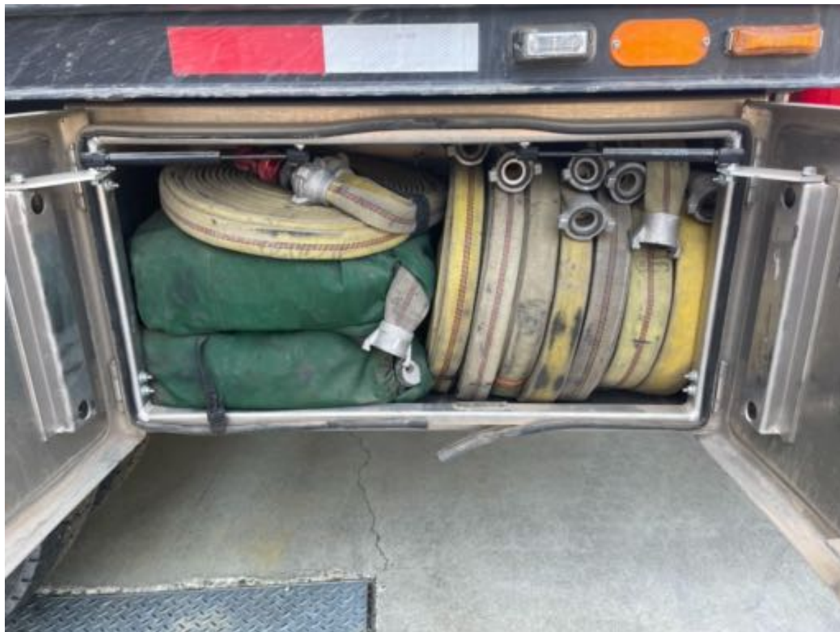
(Figure 4. One of the side boxes is for hose rolls, one roll has a nozzle pre connected for speed, the green packs are filled with two different sizes of hose as well as a nozzle and a Y valve for when the fire calls for a progressive hose lay. It is a lot funner to get the hoses out of the hose packs then get them back in)
