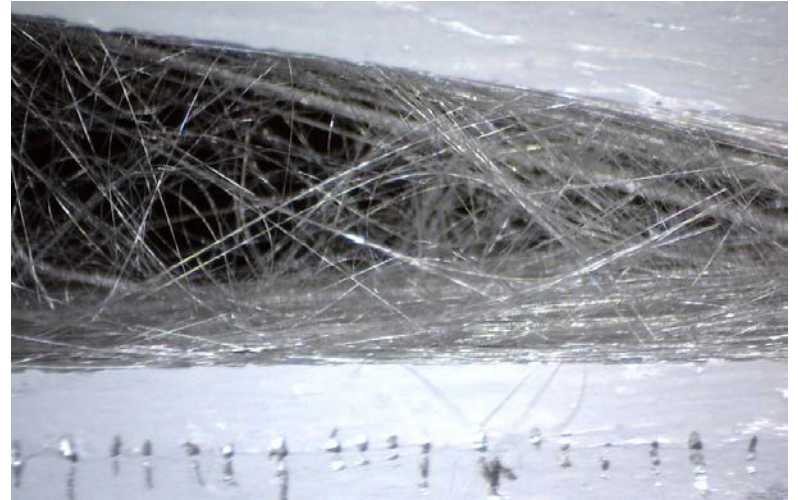
Figure 34. Fiber bridging in Plate 5 (full grind, polyester) vs Plate 3 ( \frac{1}{2} grind, vinyl ester)
