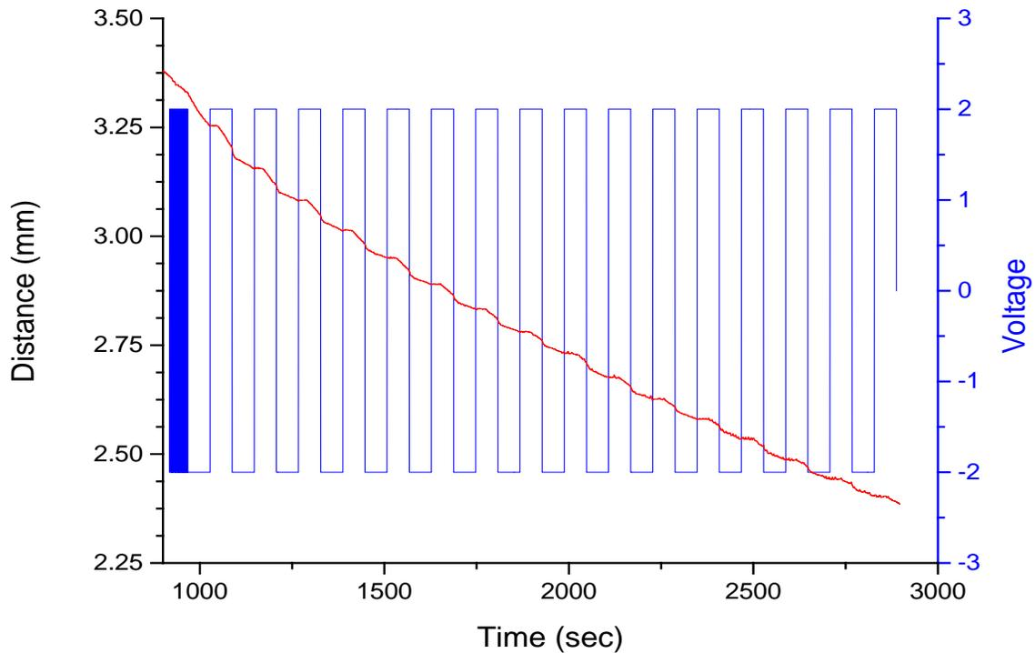
**Figure 8:** Distance (mm) and Voltage vs. Time (sec) graph from strain testing day 2 sample 3. Distance (in red) indicates the reading from the laser displacement meter during actuation (decrease in distance=elongation of actuator strip). Graph made by Nathan Bradshaw.
