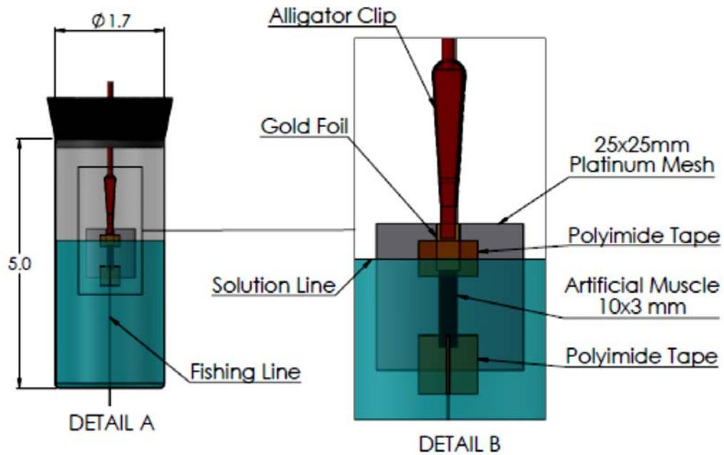
**Figure 1:** Front view of proposed solution design with close-up views of cell (Detail A) and artificial muscle assembly within cell (Detail B). Includes proposed minimum dimensions of cell and solution line.
