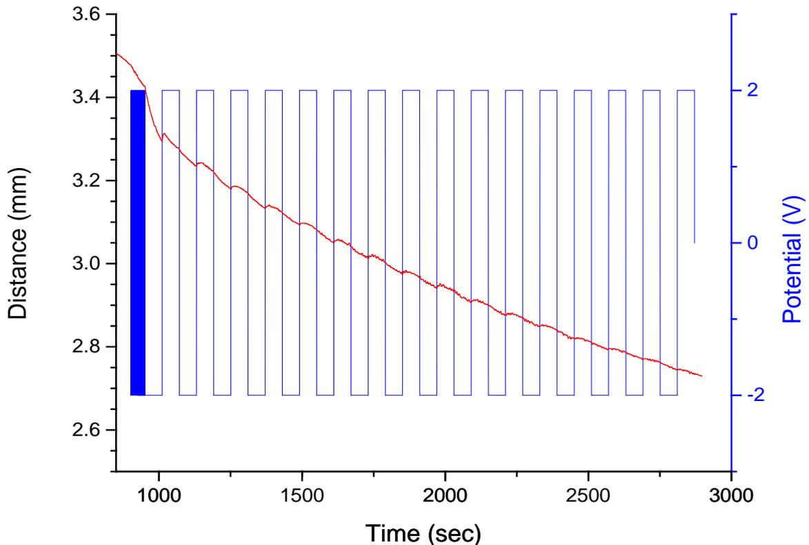
**Figure 9:** Distance (mm) and Potential (V) vs. Time (sec) graph from strain testing day 3 electropolymerized sample. Distance (in red) indicates the data from the laser displacement meter during actuation (decrease in distance=elongation of actuator strip). Graph made by Nathan Bradshaw.
