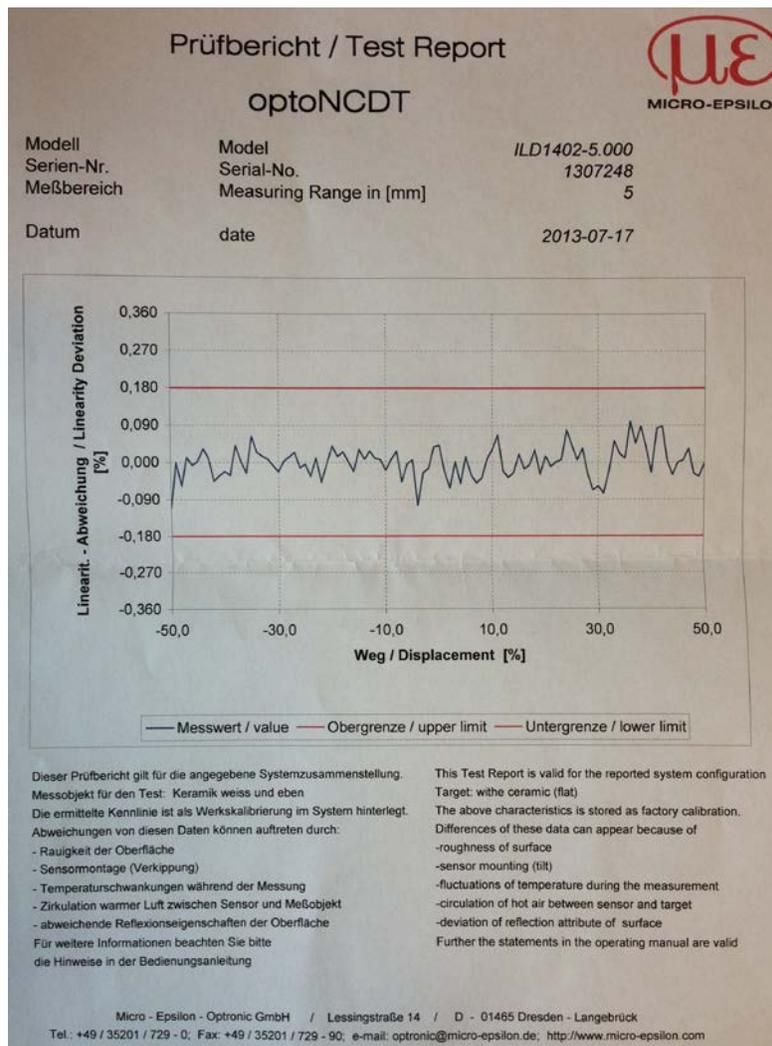
*Figure 6: Control chart sent by Micro-Epsilon showing laser was calibrated and within linearity control limits of  $\pm 0.180\%$*
