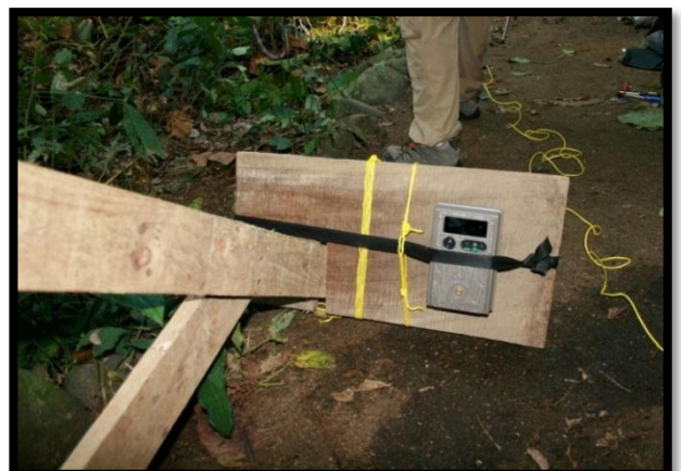
Photo 1. Camera Trap Mount.
