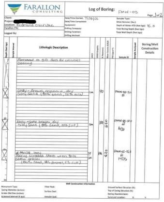
with any of the three techniques, it is Farallon's standard to remove the first five feet of soil using a vac truck to ensure that possible water lines or electrical cables are not disrupted. If they are encountered the well or boring is moved to the nearest possible position. During some projects, the location of the well may have exact coordinates. More frequently, the general location is noted, and at the discretion of the field staff, the location is finalized.
