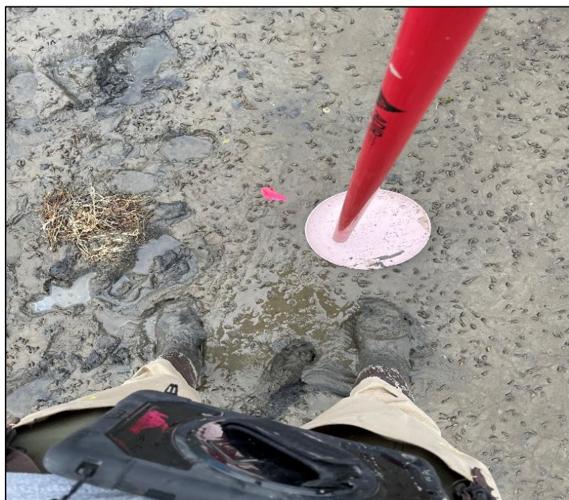
Figure 3: Photo of the pole in which an Emlid Reach (not shown) was attached to for elevation measurements. The pink plate was used to help stabilize the pole.
