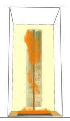
**Figure 4.** A graphic of a WFDS simulation of torching a single tree. Systematic variation of the level of defoliation and surface fire intensity allowed us to address the partial effects of defoliation on torching of individual trees.
