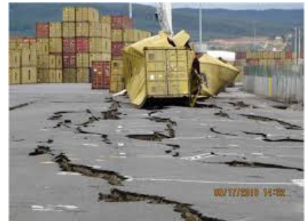
Figure 7. Damage due to liquefaction and lateral spreading at the Port of Coronel in Chile after the M8.8 Maule earthquake. Port facilities are particularly vulnerable to damage from lateral spreading. Photo: Geotechnical Extreme Events Reconnaissance (GEER).
