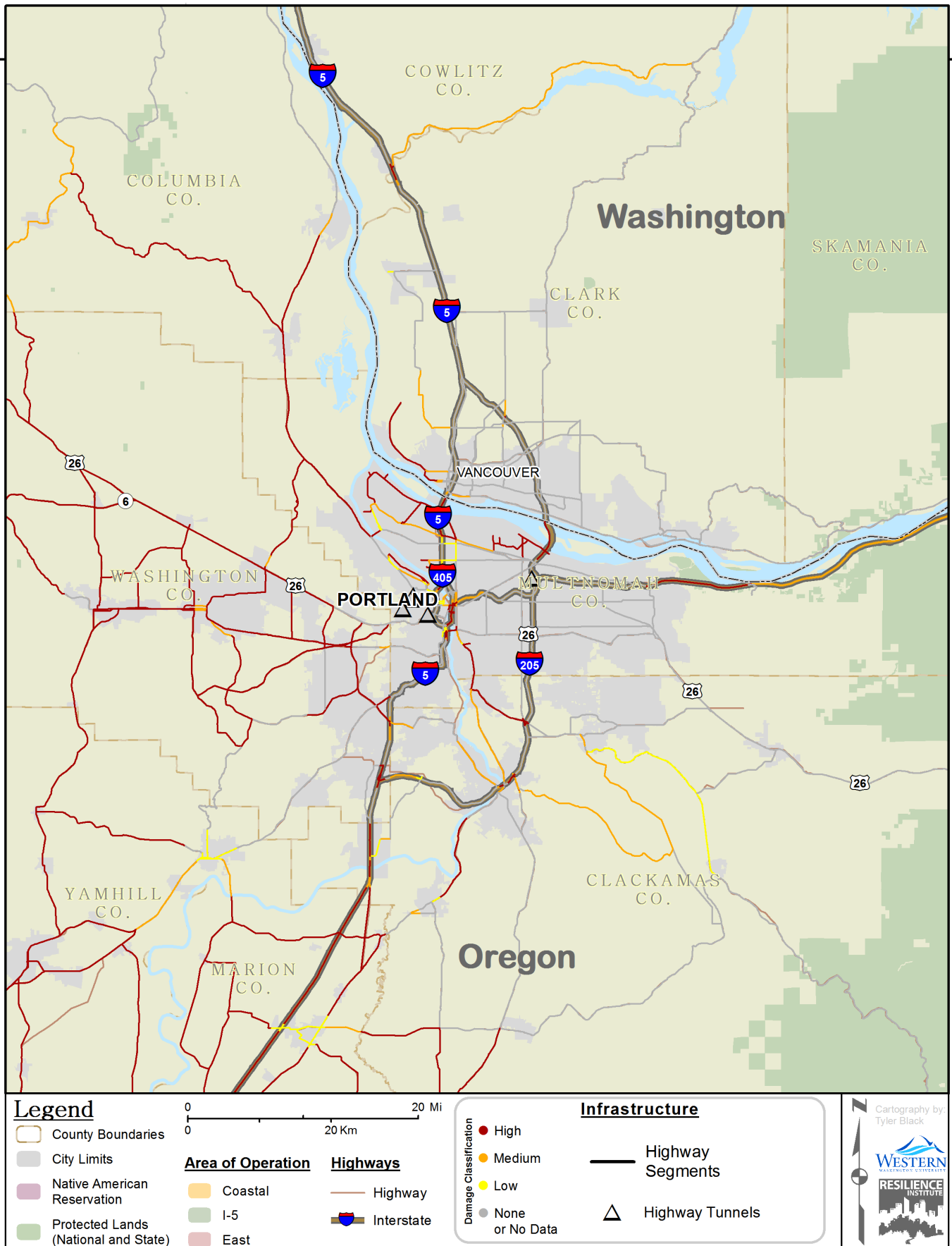
Figure 34. Road and tunnel damage on major highways in the Portland metropolitan area
