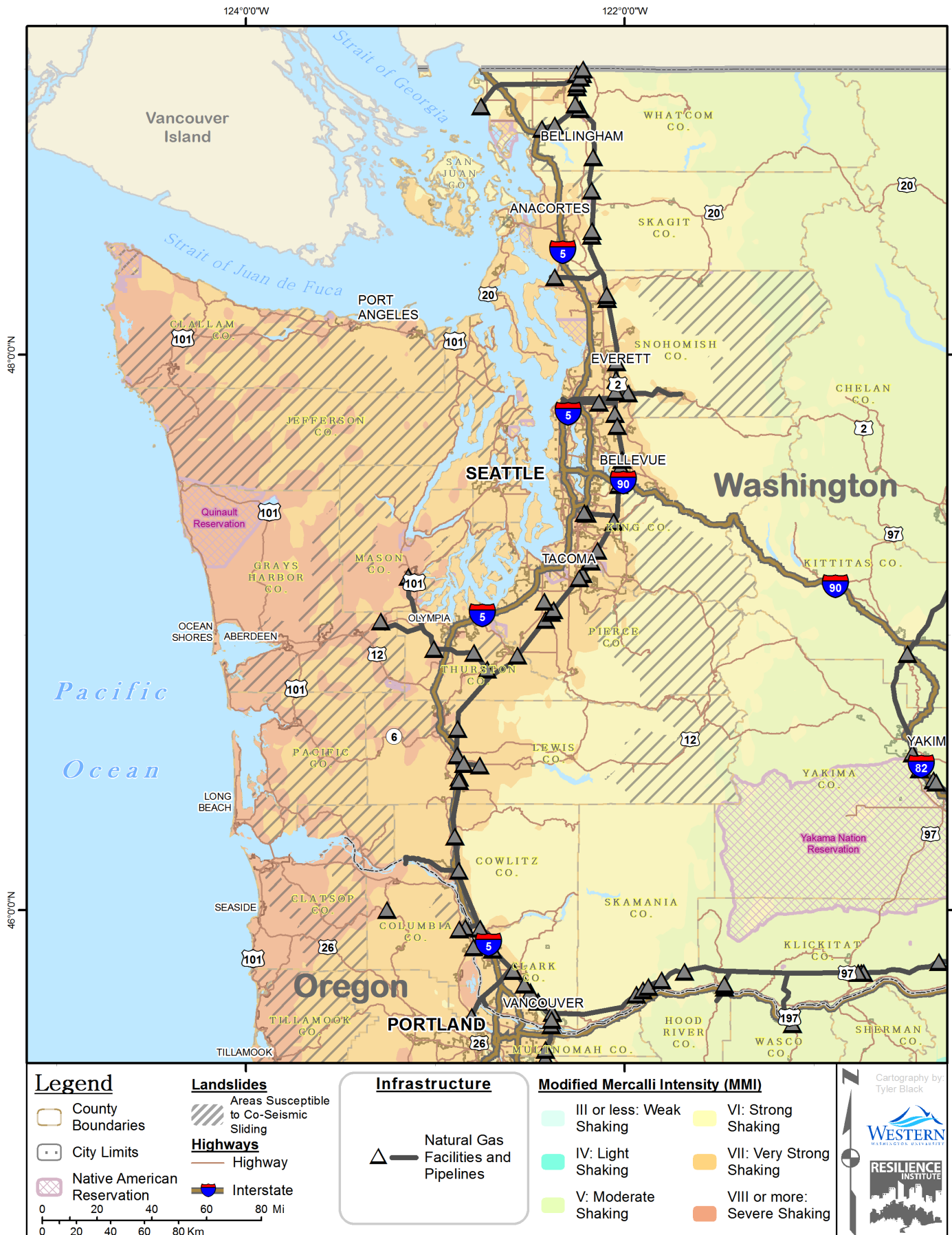
Figure 61. Washington natural gas facilities and pipelines in relation to shaking intensity and landslide potential
