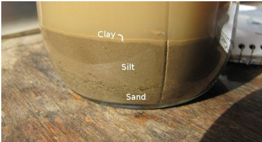
Figure 1. Layers of clay, silt and sand in a jar test photo credit: http://www.waldeneffect.org/blog/Jar_test_to_measure_soil_texture/
