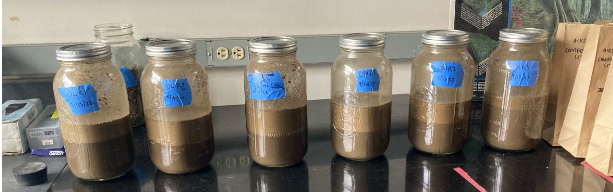
Fig. 4: Jar test setup, showing the 50/50 soil and water ratio for each jar.
