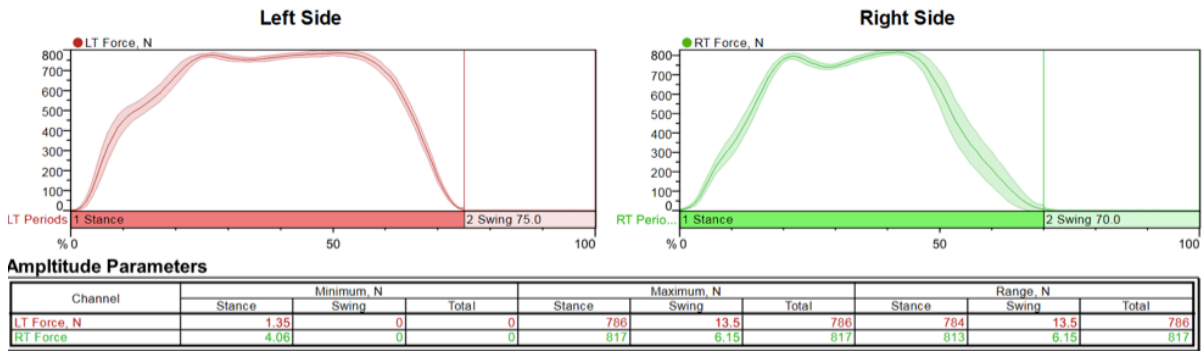
Figure 3. Vertical ground reaction force data for Subject 1 post-treatment, injured right ankle.
