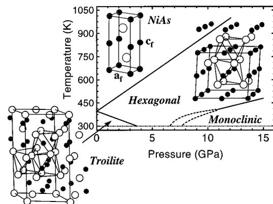
FIG. 1. Structural phase diagram of FeS derived from recent x-ray studies of Kusaba *et al.* under various  $P$ - $T$  conditions (Refs. 4 and 6). The dashed phase boundaries (6.5–7.5 GPa) demarcate a range where two phases coexist. Straight solid lines in the structures show the unit-cell as well as the octahedral coordination of Fe (small shaded circles) by S (larger open circles) atoms.
