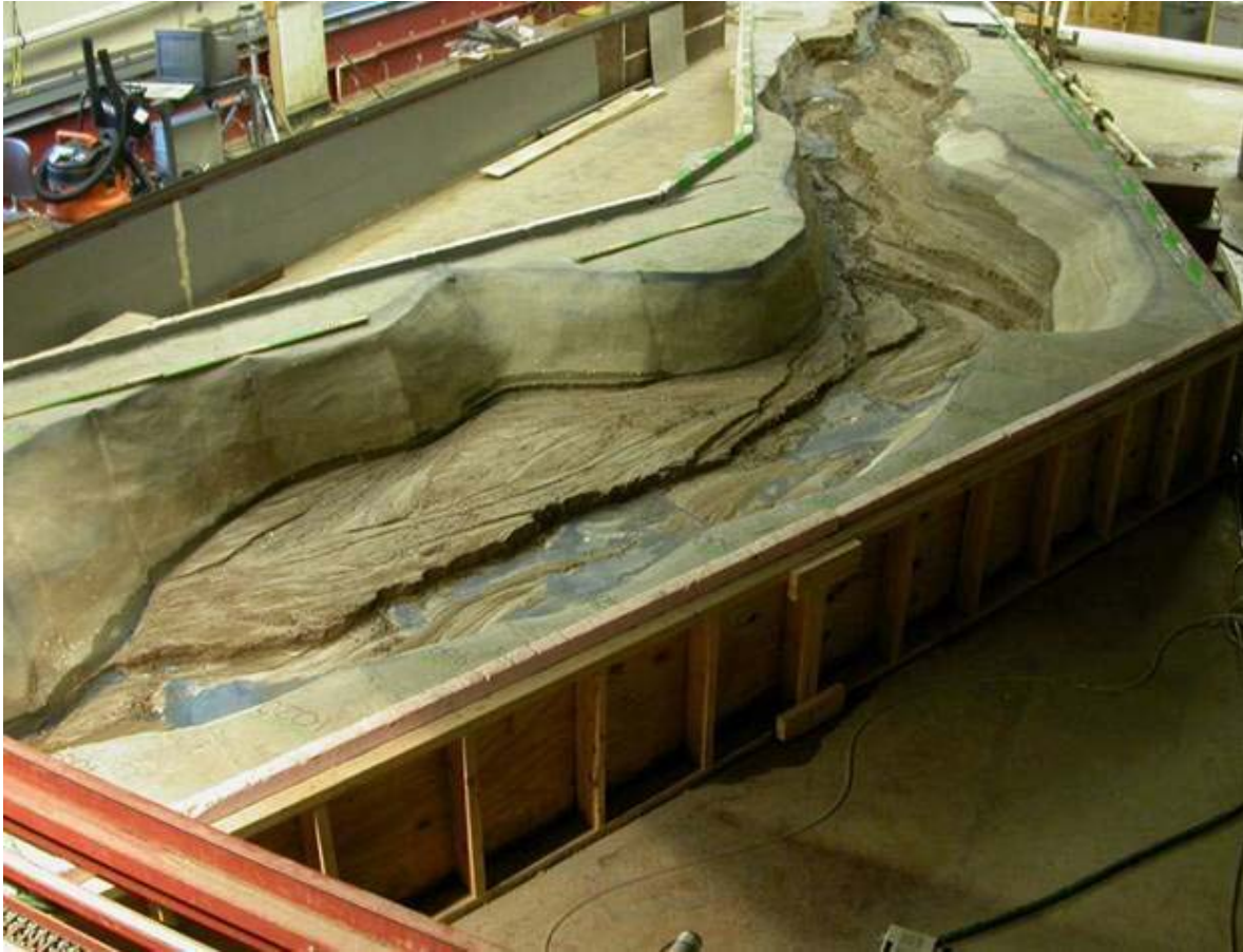
FIGURE 2. Scale model of Lake Mills depicting terracing of sediments left behind following dam removal (Reproduced with permission of C. Bromley).
