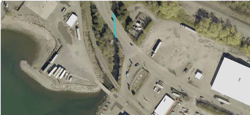
Figure 2.5: City of Bellingham Sewer Line Location. The blue line represents the location of the City of Bellingham sewer main under Squalicum Creek. The blue line also represents the length of concrete lining the bottom of the creek to be removed under the proposed and alternative action.
