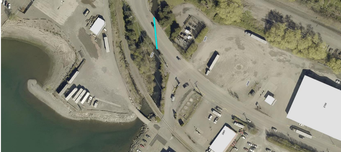
Figure 4.3: City of Bellingham Sewer Line Location. The blue line represents the location of the City of Bellingham sewer main under Squalicum Creek. The blue line also represents the length of concrete lining the bottom of the creek to be removed under the proposed and alternative action. (CityIQ for City of Bellingham)
