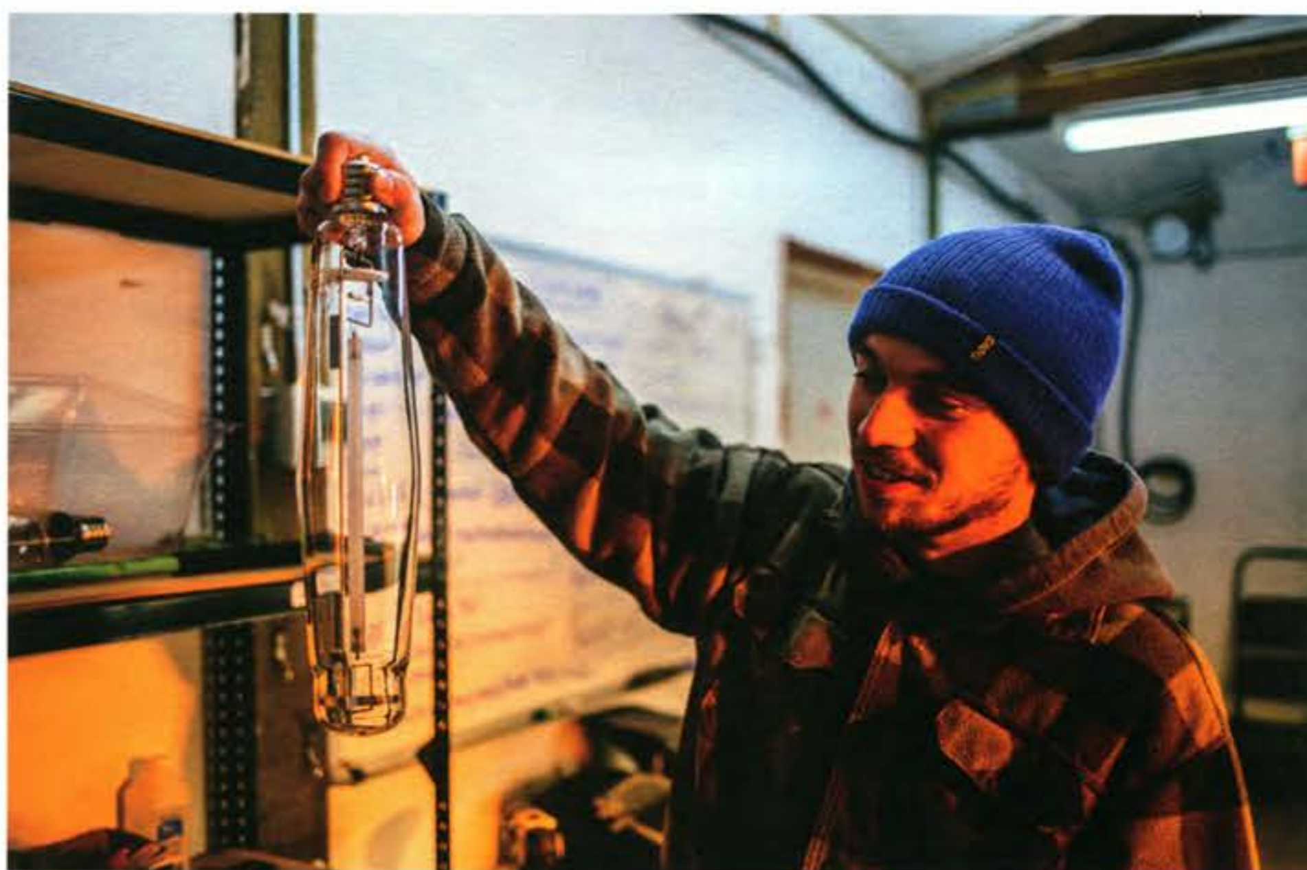
ABOVE: Trent Prengel holds an old high-intensity discharge (HID) bulb. His grow operation recently upgraded to more efficient and longer-lasting Gavita grow lights.
