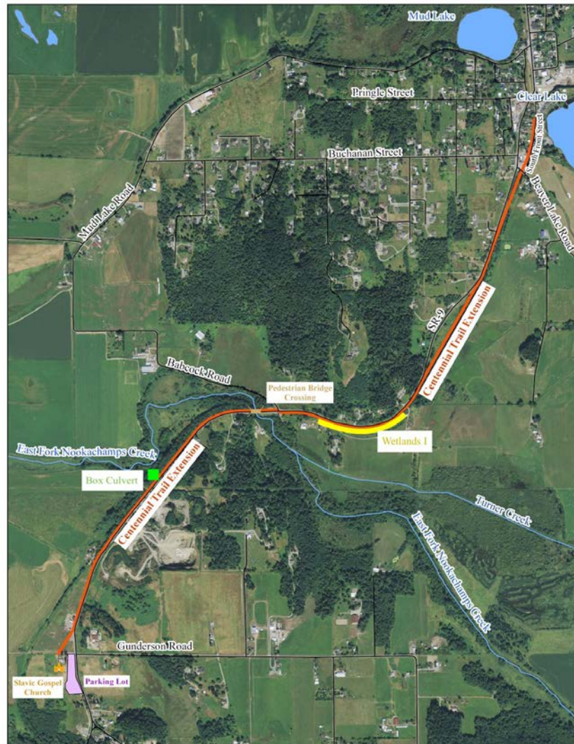
Figure 4. Intersection of the Centennial Trail extension and adjacent water bodies. The three water crossings are depicted as follows: Wetlands I (yellow), East Fork Nookachamps Creek (tan pedestrian bridge), and the box culvert (green). Data sources: Sam Kaiser and WWU 2018.
