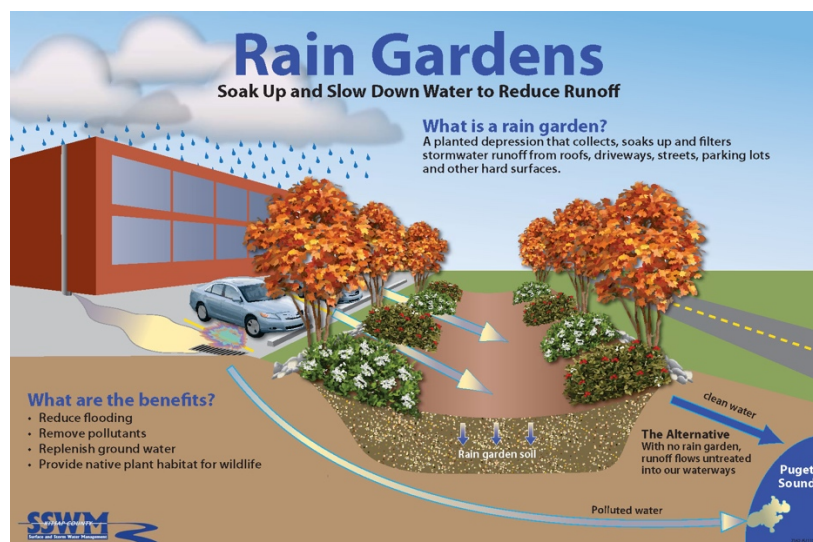
Figure 13. Rain Garden Diagram (Center for Sustainable Infrastructure, 2015)
