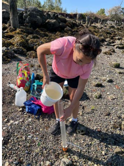
Figure 2: Measuring turbidity with a turbidity tube at the Cedar St. outfall during a stormwater sampling event.
