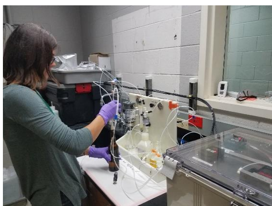
Figure 3. Analysis of carbonate samples on the Burke-o-lator, a carbonate chemistry analyzer.
