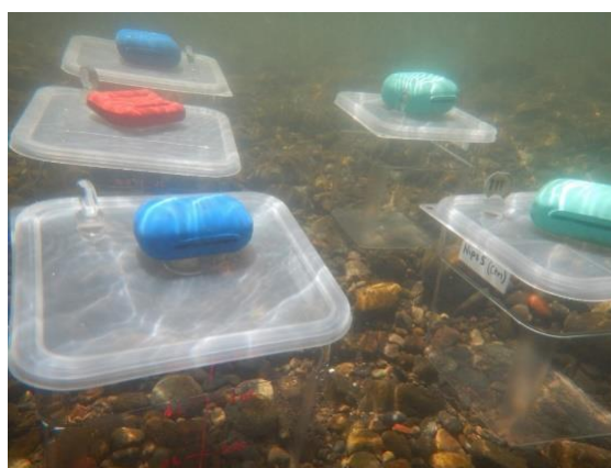
Figure 4. Sealed microcosm chambers (light treatment) placed in the Trask River to measure in-stream processing
