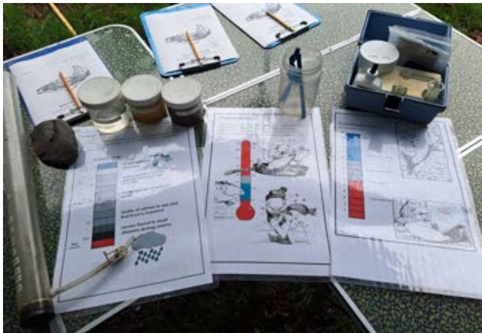
Figure 5. This image depicts the posters and materials used for the water quality station. On the left is a turbidity tube and the three jars with various degrees of turbidity along with the poster explaining how salmon are affected by different turbidity levels. In the center is the jar and thermometer used to measure the stream temperature and the poster for optimal water temperature for salmon. On the right is the hatch kit with all the supplies to measure dissolved oxygen and the poster showing how much oxygen salmon need.
