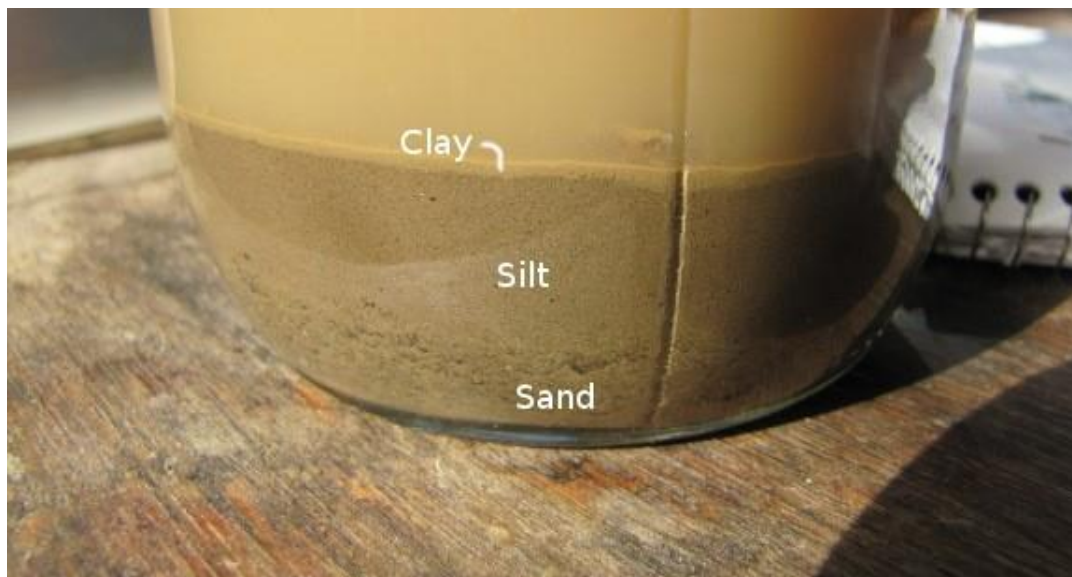
Figure 6. Layers of clay, silt and sand in a jar test (Anna).
