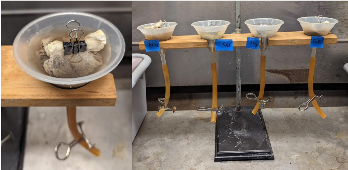
Figure 4. Nematode extraction set up using the Baerman funnel technique.
