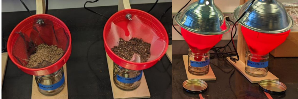
Figure 5. Microarthropod extraction set up using the Tullgren funnel technique.
