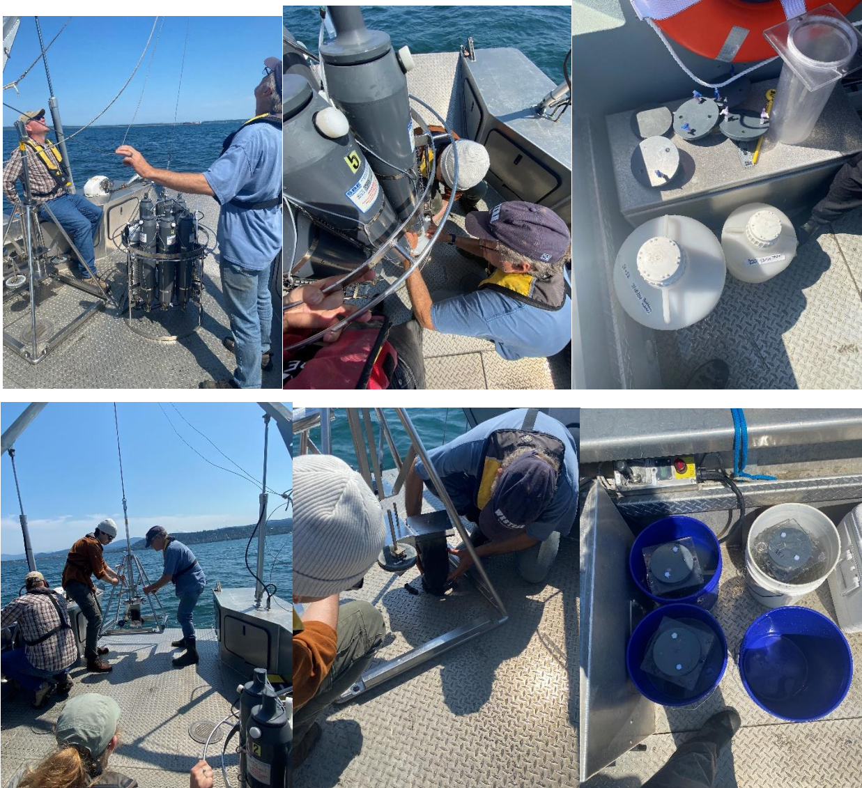
The CTD being prepared to be lowered into the water at Site 1 (upper left). Water samples being taken from the CTD at Site 1 with canisters labeled Site 1 and 2 (upper middle). Canisters that will be filled with water from the CTD, a sediment core tube, and caps for the sediment cores (upper right). The Haps Corer being lifted back onto the boat after taking a sediment core; see the dark tube in the middle of the device filled with mud from Site 2 (lower left). The sediment core being unloaded from the Haps Corer at Site 2 (lower middle). The sediment cores sitting in ice baths to maintain sea bottom temperatures for the journey back to the lab (lower right).
