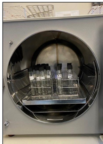
Figure 4: Processed total phosphorous and nitrogen sample aliquots in the autoclave.
