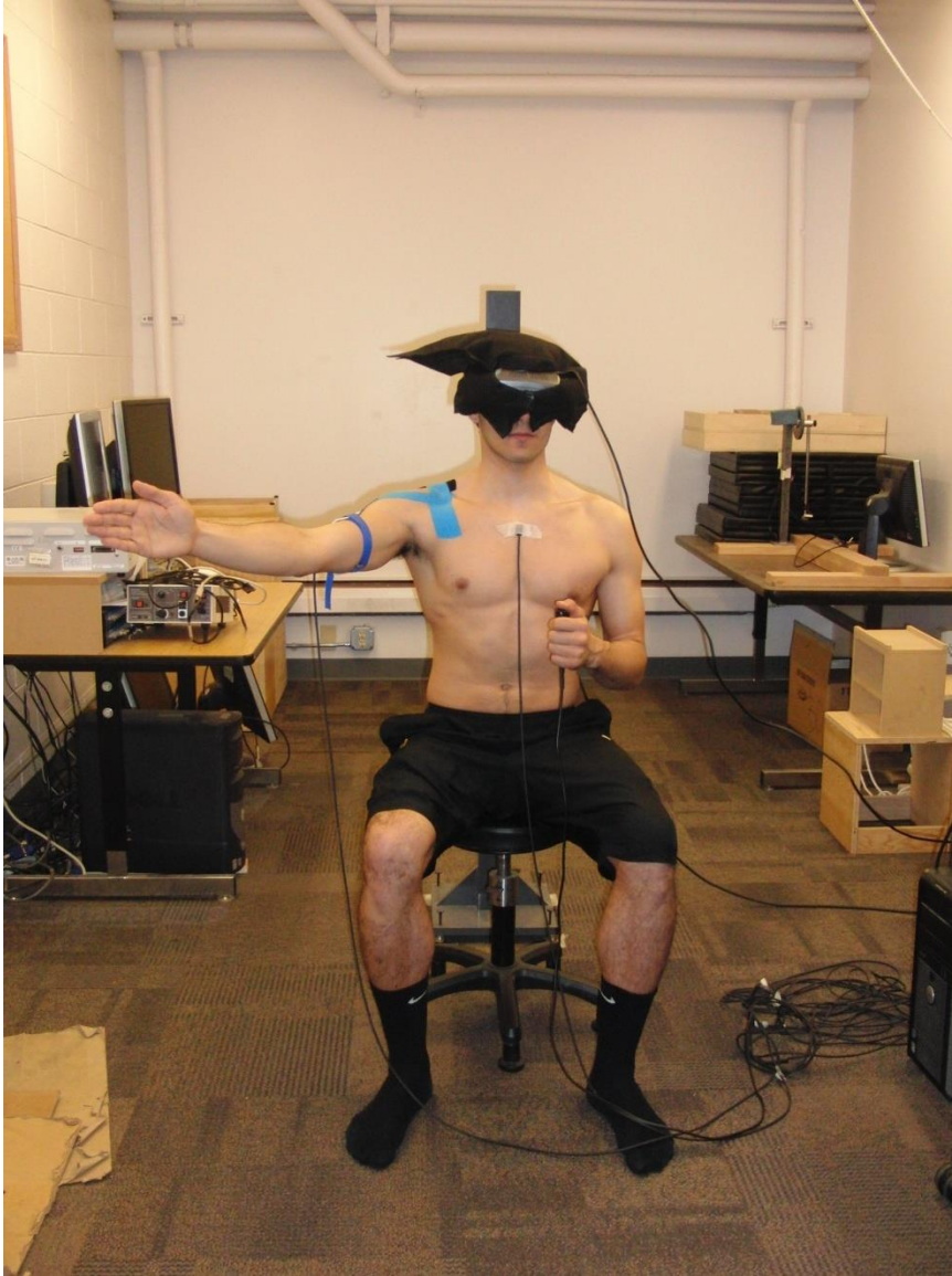
Figure 4. Experimental set-up showing, sensors, head-mounted display and kinesio tape.
