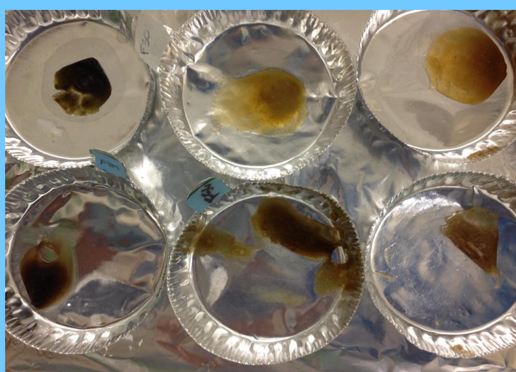
Figure 6. Alginate dried overnight in an oven at 50°C.
