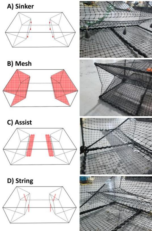
**Figure 2.** This image shows mechanical adjustments to the Fukui trap to aid in *C. maenas* entry and capture. **A.** Three sinkers attached to the bottom edge of the entry slit to weigh it open. **B.**
