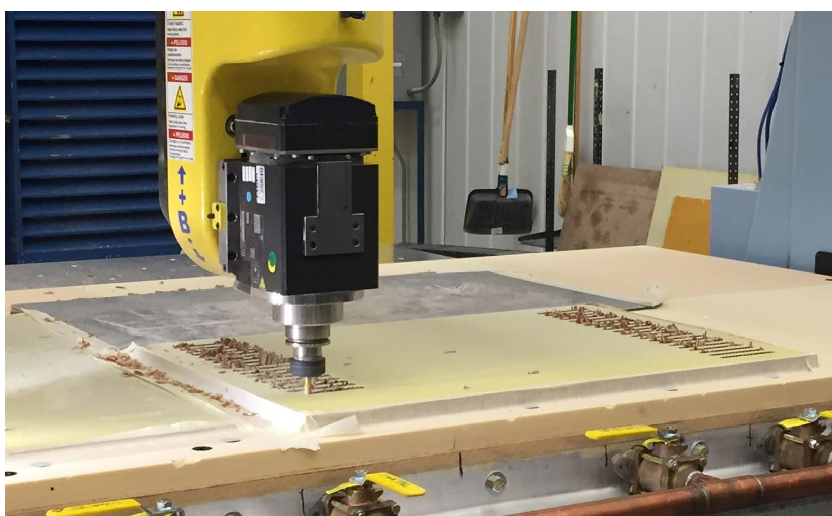
Panel machining with CNC router at Zodiac
