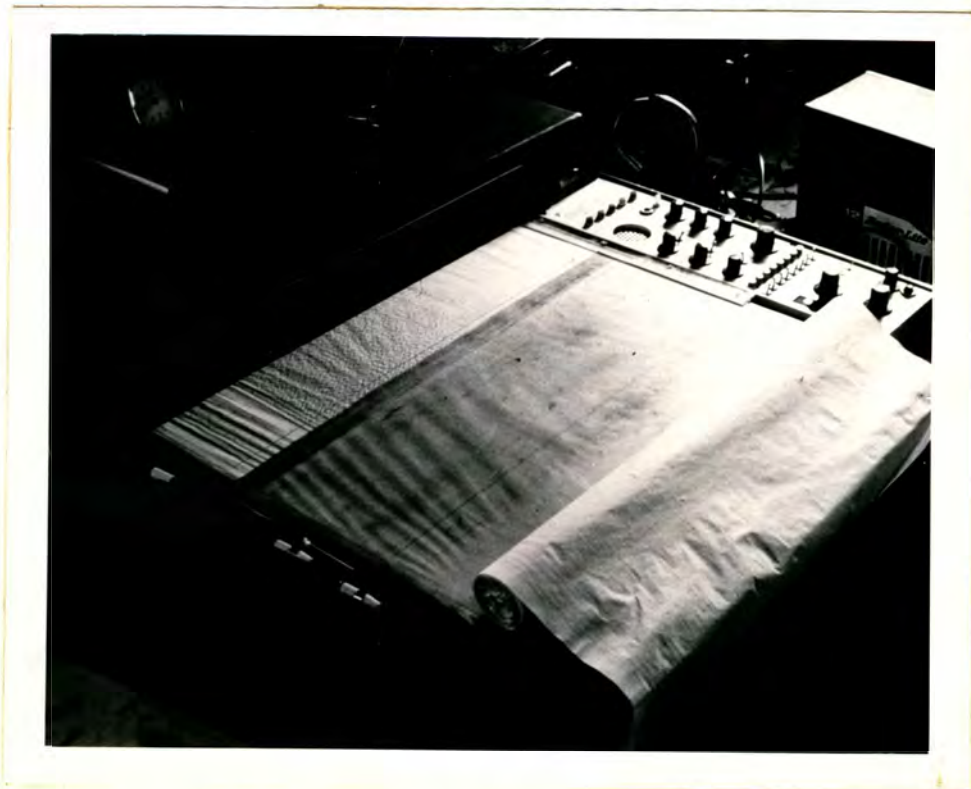
Fig.4 Sub-bottom profile recorder in operation.
