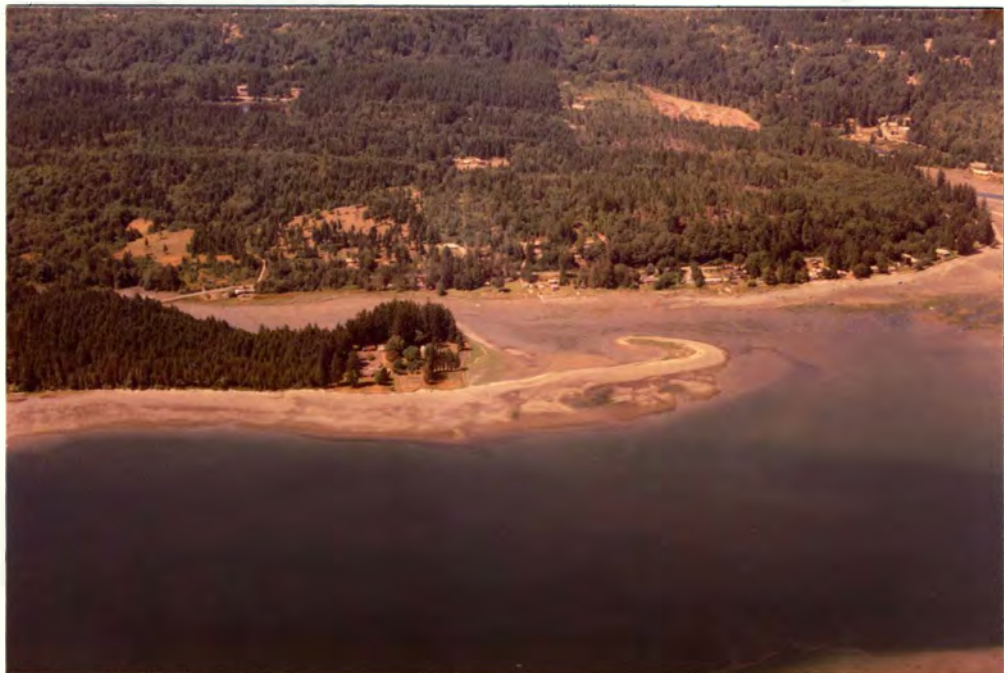
FIGURE 26: Northward growth (toward right) of this spit at Wilson Point, Hartstene Island, occurs because of change in shoreline orientation relative to predominant wave direction. Photo taken from 300 m altitude.
