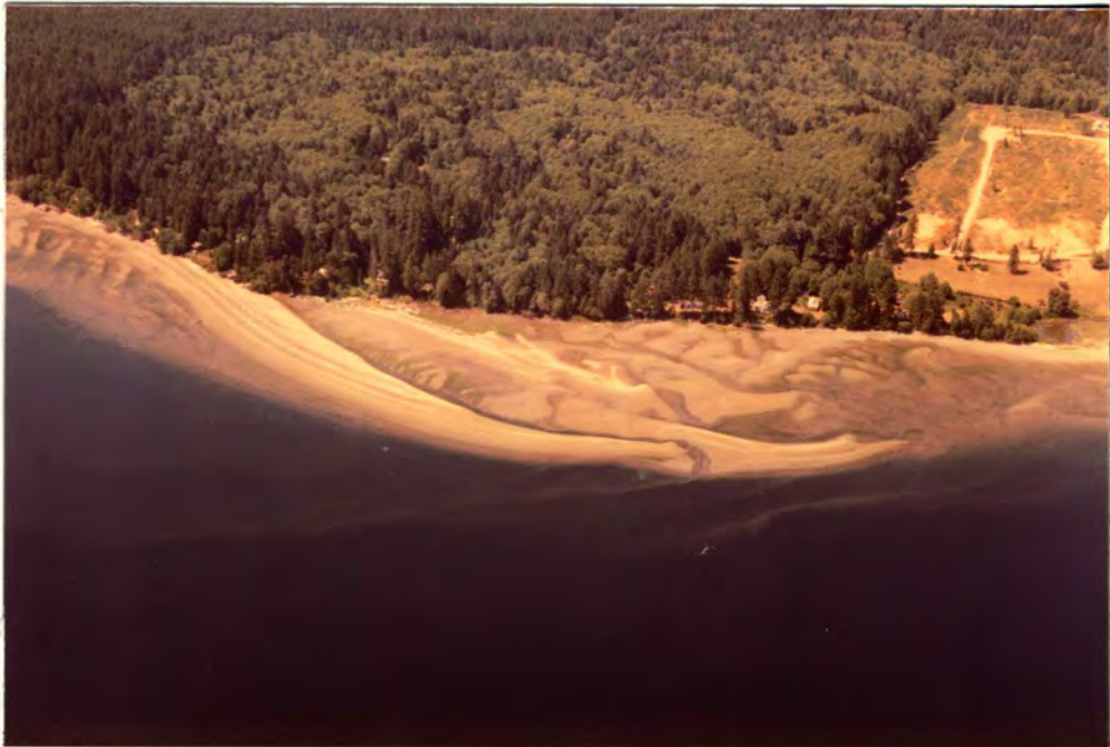
FIGURE 26: Northward growth (toward right) of this spit at Wilson Point, Hartstene Island, occurs because of change in shoreline orientation relative to predominant wave direction. Photo taken from 300 m altitude.
