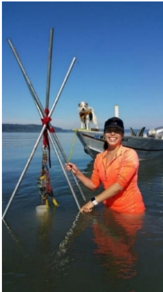
Figure 4: Field team, Erin Murray, University of Washington, and Taz, sediment coring with 10 cm x 1.4 m pvc coring tubes, aluminum tripod, and come-along in Skagit Bay, Wa.
