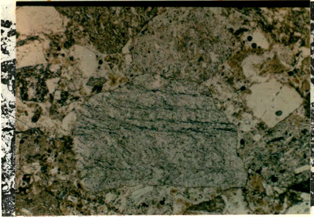
Figure 62.a. Recrystallized and deformed chert grain. Sample 32-12-25-1. Field of view 2.1 x 1.5 mm. Plain light.
