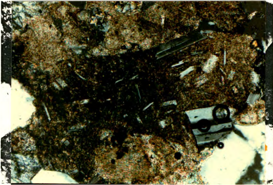
Figure 38. Volcanic lithic being altered to calcite. Sample 32-11-32-6. Field of view .85 x .58 mm.
