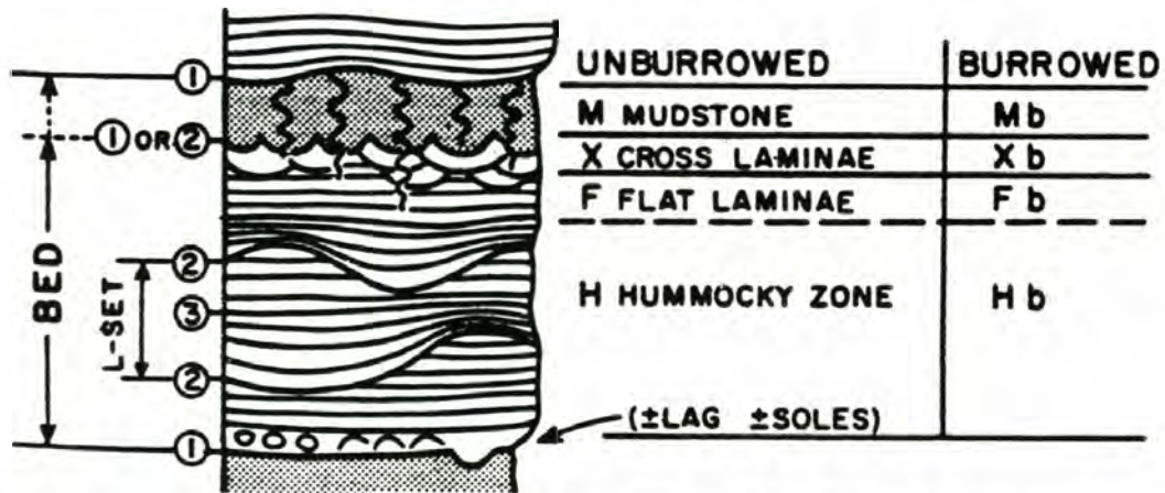
Figure 19; The idealized hummocky cross stratified sequence comprised of the various component zones. From Dott and Bourgeois, 1982.
