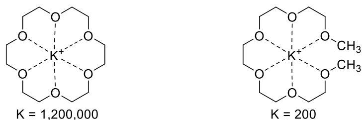
Figure 3.1. Binding constant of K^+ 18-crown-6 (left) and pentaethylene glycol dimethyl ether in dry MeOH.
