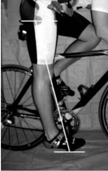
Figure 4. Seat height measured at crank BDC 37
