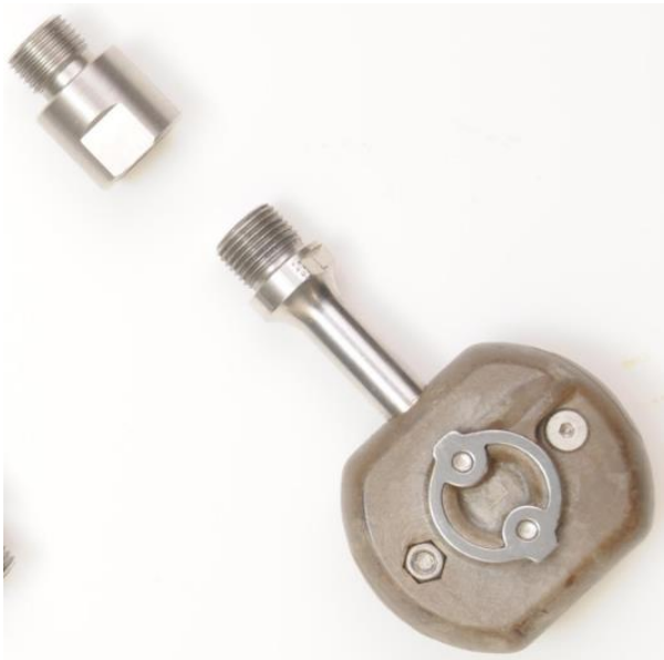
Figure 10. Kneesavers™ Pedal spacers effectively extend pedal width by increasing distance from crank to pedal centerline. 47
