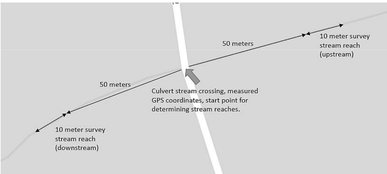
Figure C.1. Diagram showing the general configuration of a field site. The culvert stream passage was noted using GPS coordinates. Upstream and downstream survey sites were found by traveling 50 meters from the culvert in each direction and demarcating a 10-meter stream reach for variable and salamander sampling. Map data: Google, 2020.
