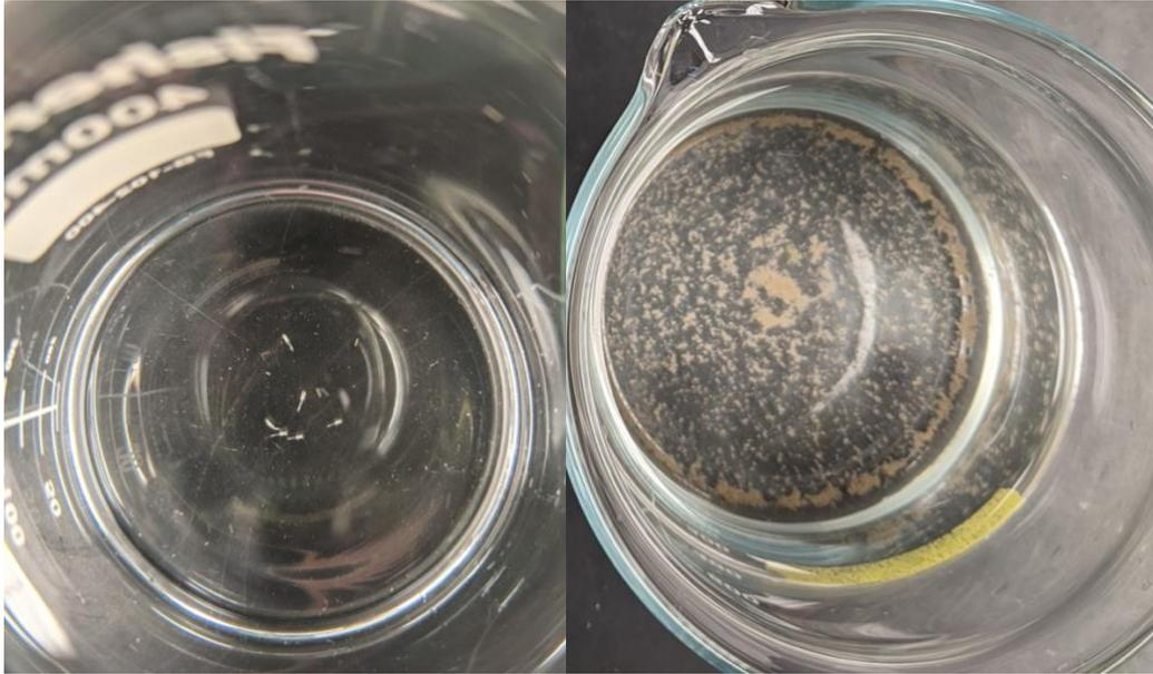
**Figure 6.** Photo of a toxicity test beaker filled with leachate from an unaged microplastic (left) versus a test beaker filled with aged microplastic leachate (right). Note the  $<10\ \mu\text{m}$  sediments that have settled to the bottom of the right test chamber, which made it through the two filter screens used to process all leachates.
