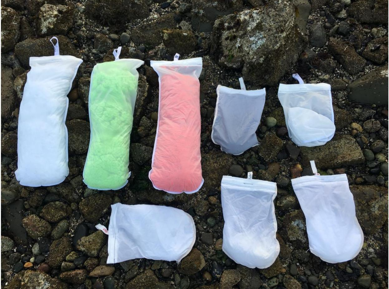
**Figure 4.** Microplastic particles and fibers contained in 10 µm nylon monofilament filter bags immediately before deployment in Bellingham Bay, WA. Bags were sewn closed at the top and fabric loops included to allow attachment to an anchor setup.
