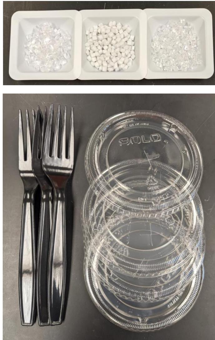
**Figure 1.** Five plastic types prior to grinding into microplastic particles in a Blendtec blender. The top row includes (from left to right) virgin polystyrene, virgin polyethylene terephthalate, and virgin polycarbonate. The bottom row includes (from left to right) consumer polystyrene as black disposable forks, and consumer polyethylene terephthalate as disposable cup lids.
