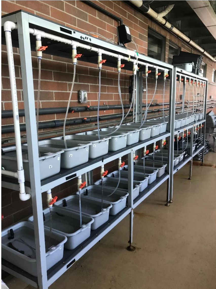
Figure 1. Flow through sea water system setup for feeding trial experiment with totes (n=24). 18 different sea cucumbers were placed into 18 totes and fed a randomized diet of either mussel biodeposits, dulse, or a 50:50 mix of the two diets. 6 totes were used as controls. After 48 hours, bins and sea cucumbers were rearranged and a new food treatment was fed to the same sea cucumbers. All treatments shared water supplied from the same inlet.
