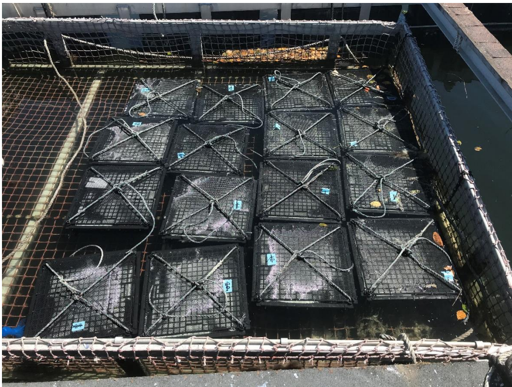
Figure 2. Enclosure design used for in situ experiment. Tyvek walls extended 8 cm from the bottom of cages to capture sediments.
