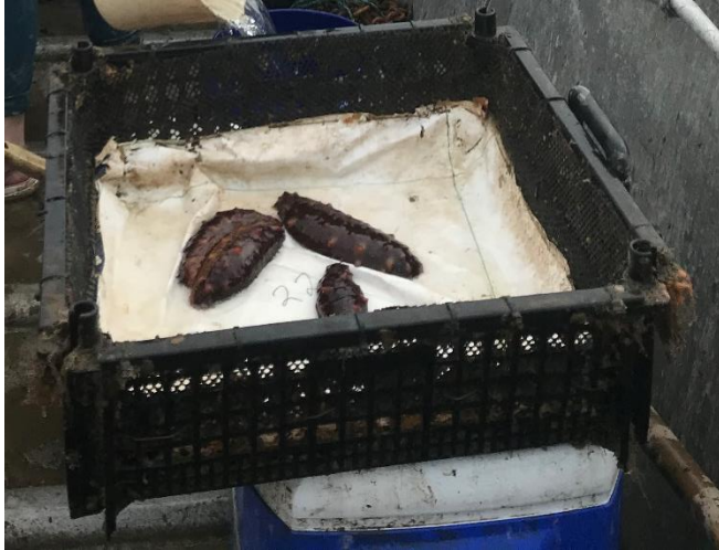
Figure 2. Enclosure design used for in situ experiment. Tyvek walls extended 8 cm from the bottom of cages to capture sediments.
