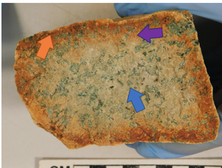
Figure 4: Photo of a Twin Sisters dunite sample with a bright orange weathered exterior (orange arrow) and a relatively unaltered green interior (blue arrow). An approximately 2 cm thick gradient between the two is present (purple arrow).
