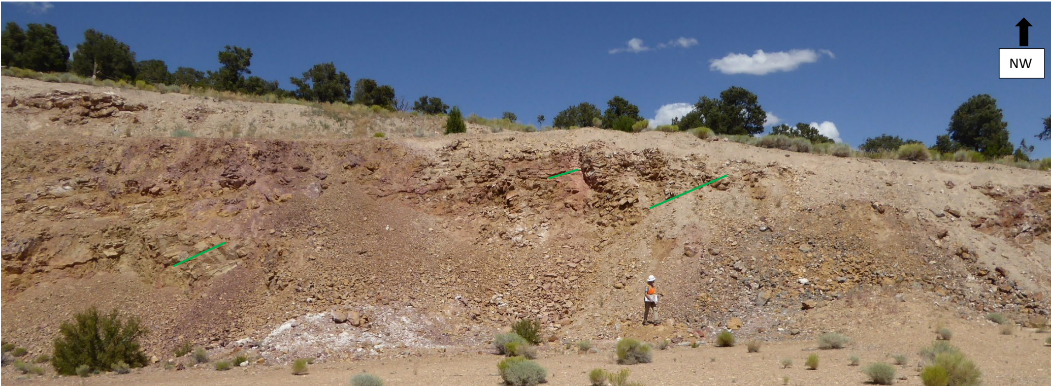
Figure 36-Looking northwest, photo of the upper benches of the west wall of the Royale West pit showing moderately west-dipping beds of Dg limestone. Location of photo shown in Figure 33. Photo by Liz Schermer.
