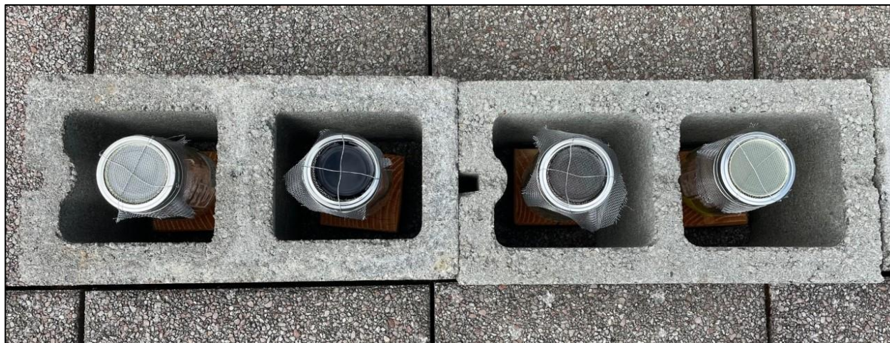
Figure 3. Outdoor weathering experimental setup utilized 16-ounce Mason jars with galvanized steel wire and mesh lids stabilized within cinderblocks on the roof of the Environmental Studies building at Western Washington University.
