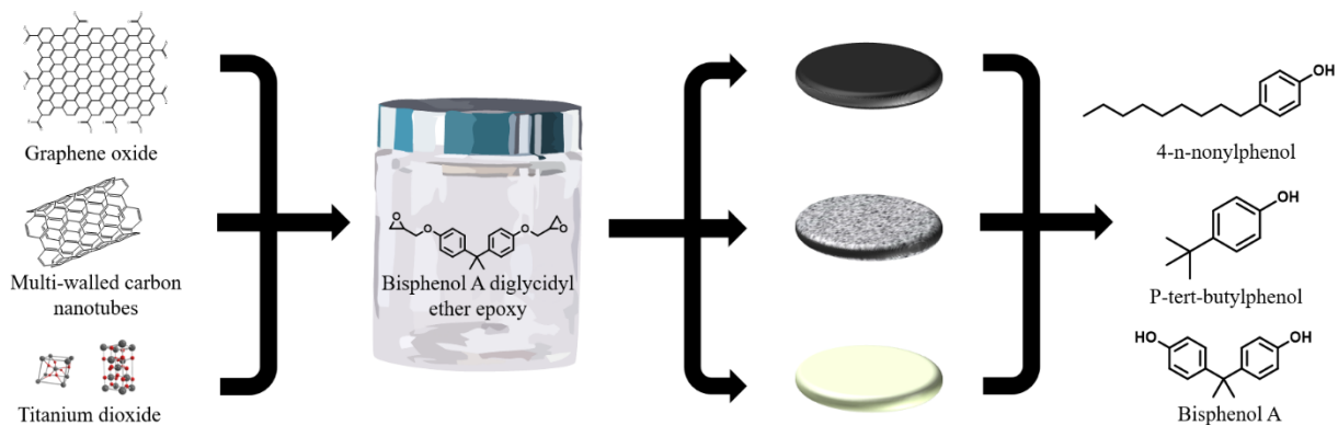
Figure 1. Experimental design of PNC leaching experiments involved the inclusion of NMs in BADGE epoxy and quantification of additive release in leachate using HPLC-QTOF-MS.
