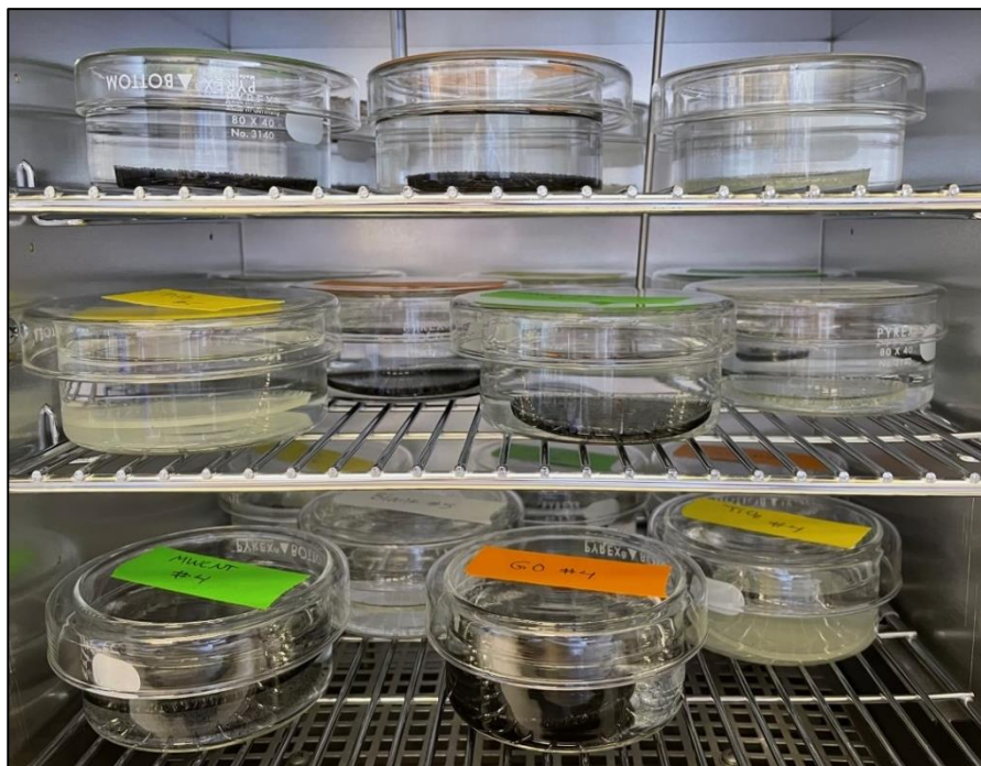
Figure 2. Glass crystallizing dishes each containing one PNC and 100 mL of EPA MHW were placed in a drying oven at room temperature, 45°C, or 65°C.
