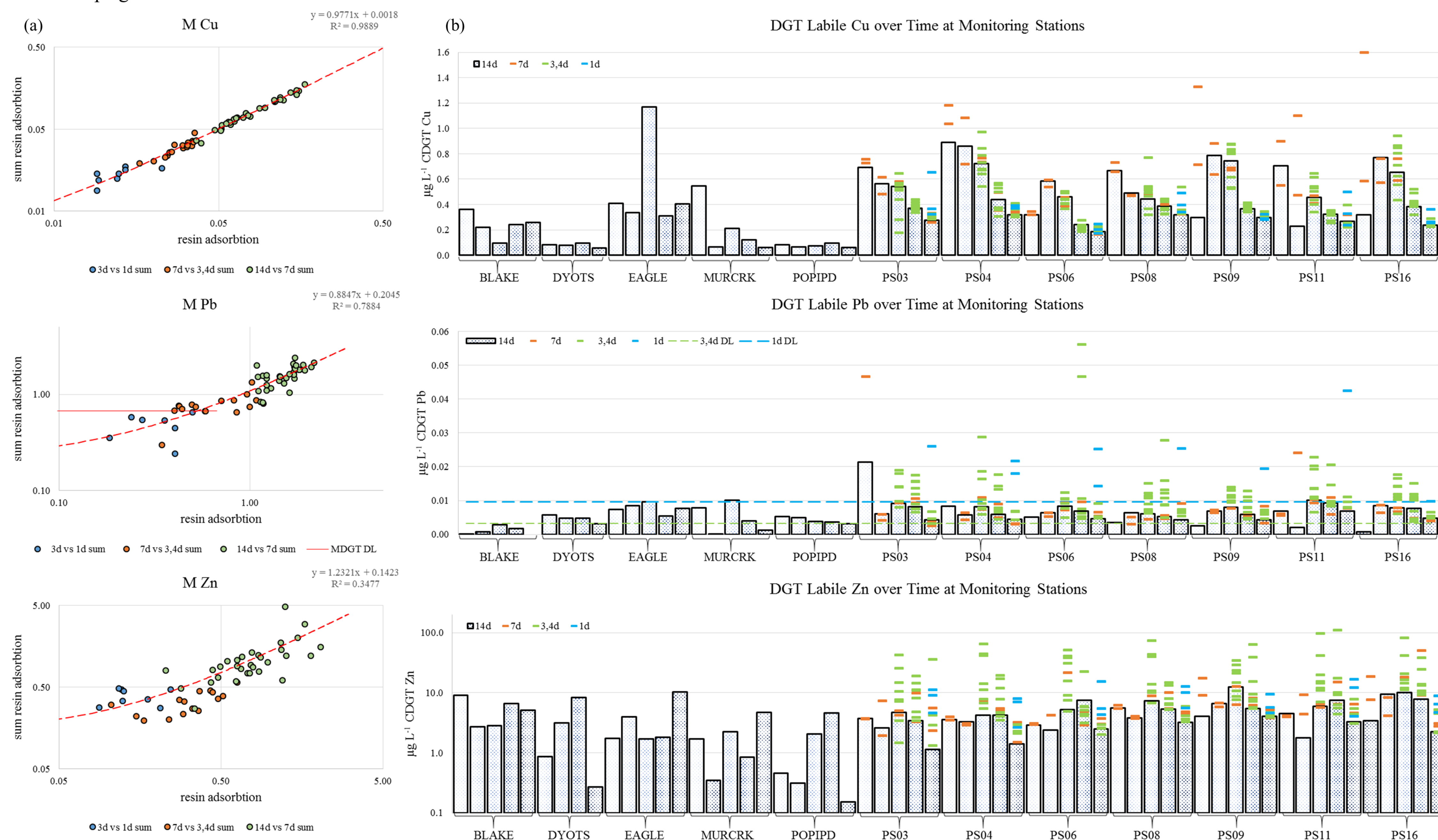
Figure 3. (a) Analyte sensitivity when moving from 14 days to 1 day deployment time, displayed as M (metal resin -1 ) ( n 1-day = 24; n 3, 4, and 14-day = 32; n 7-day = 64); (b) CDGT at monitoring stations during 5 campaigns (03/07/16-03/23/16; 08/24/16-09/08/16; 11/28/16-12/12/16; 03/16/17-03/29/17; 08/16/17-08/29/17), where 14 day CDGT is signified by bars grouped by station and chronological from left to right. Colored lines represent variation captured at sub 14 day times within the 14 day period.
