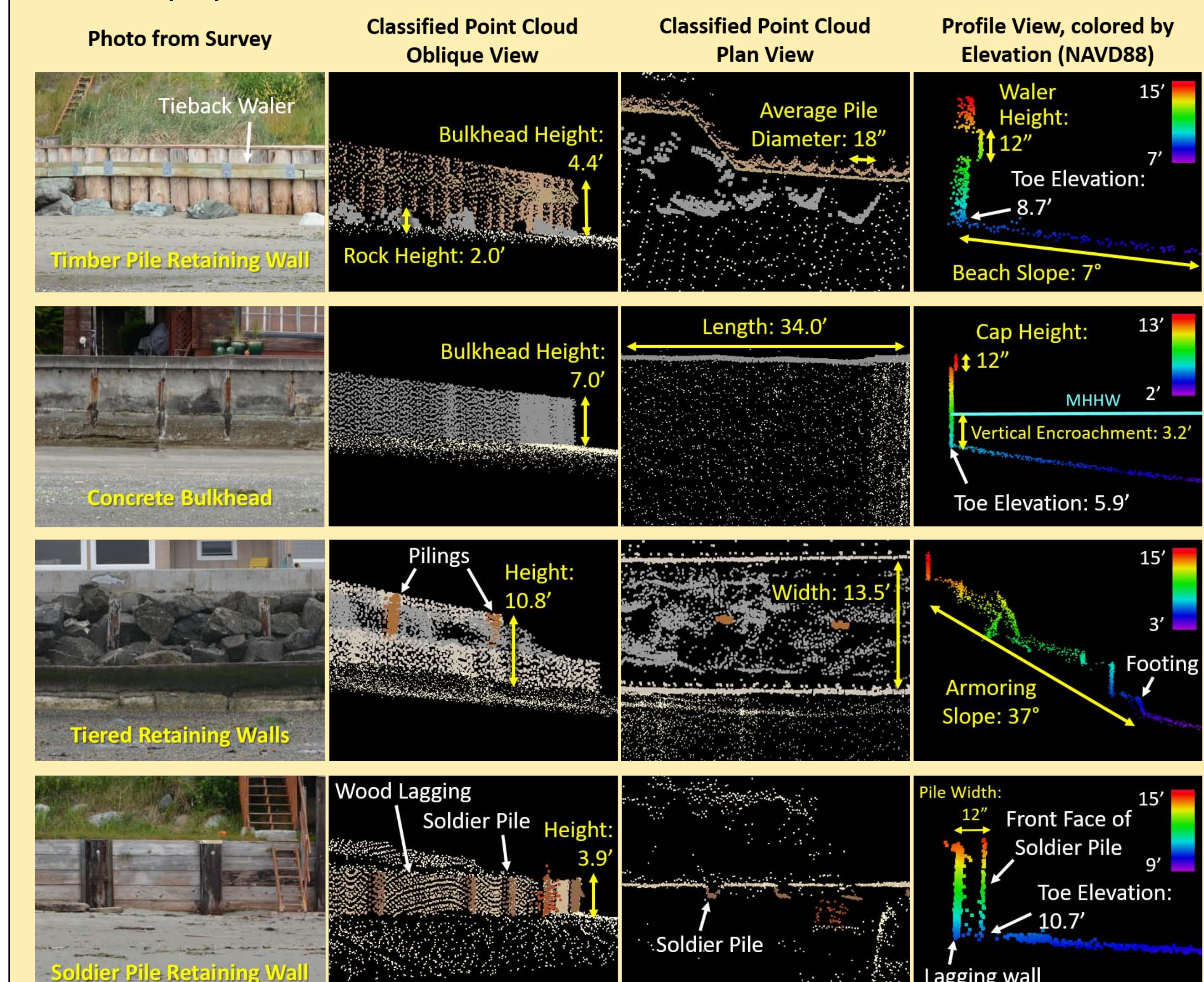
The combination of high-resolution point clouds and photos from field surveys enables the identification and measurement of a wide variety of shoreline modifications.
