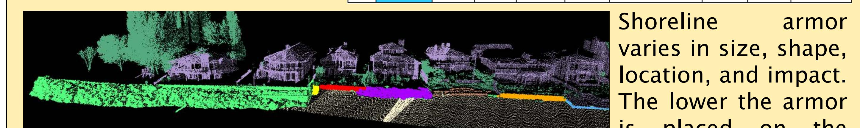
Shoreline armor varies in size, shape, location, and impact. The lower the armor is placed on the beach, the more it impacts nearshore processes, structure, and functions.
