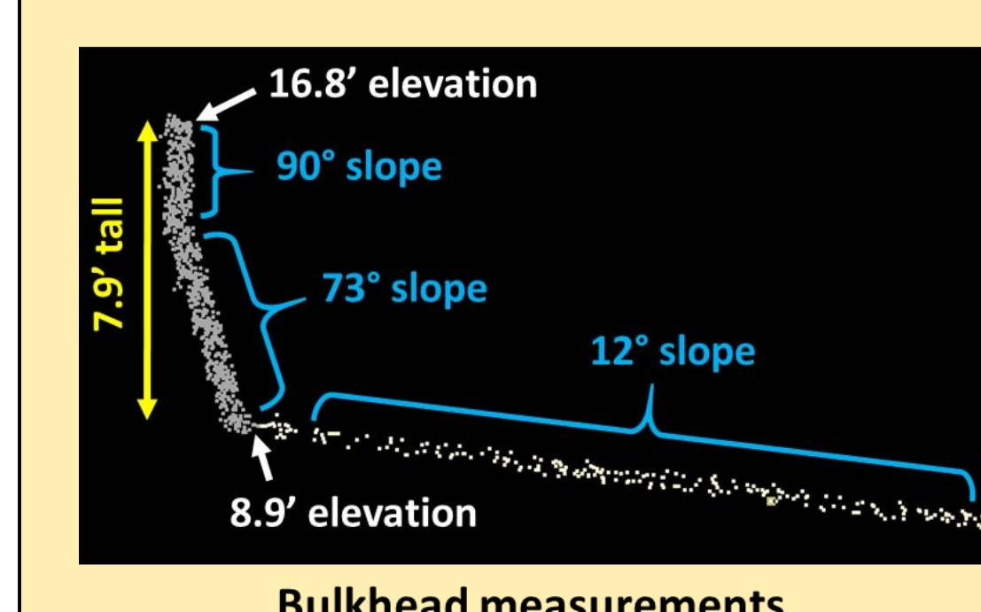
Accurate quantification and inventory of Puget Sound shoreline armor is crucial for assessment of impact and restoration opportunities. The high-resolution point clouds allow detailed mapping of shoreline armor attributes such as type, length, elevation, height, slope, and condition within the context of shoreform and beach morphology. The point cloud inventory of armor attributes allows for precise measurement and change detection that is accurately georeferenced in 3D map space.
