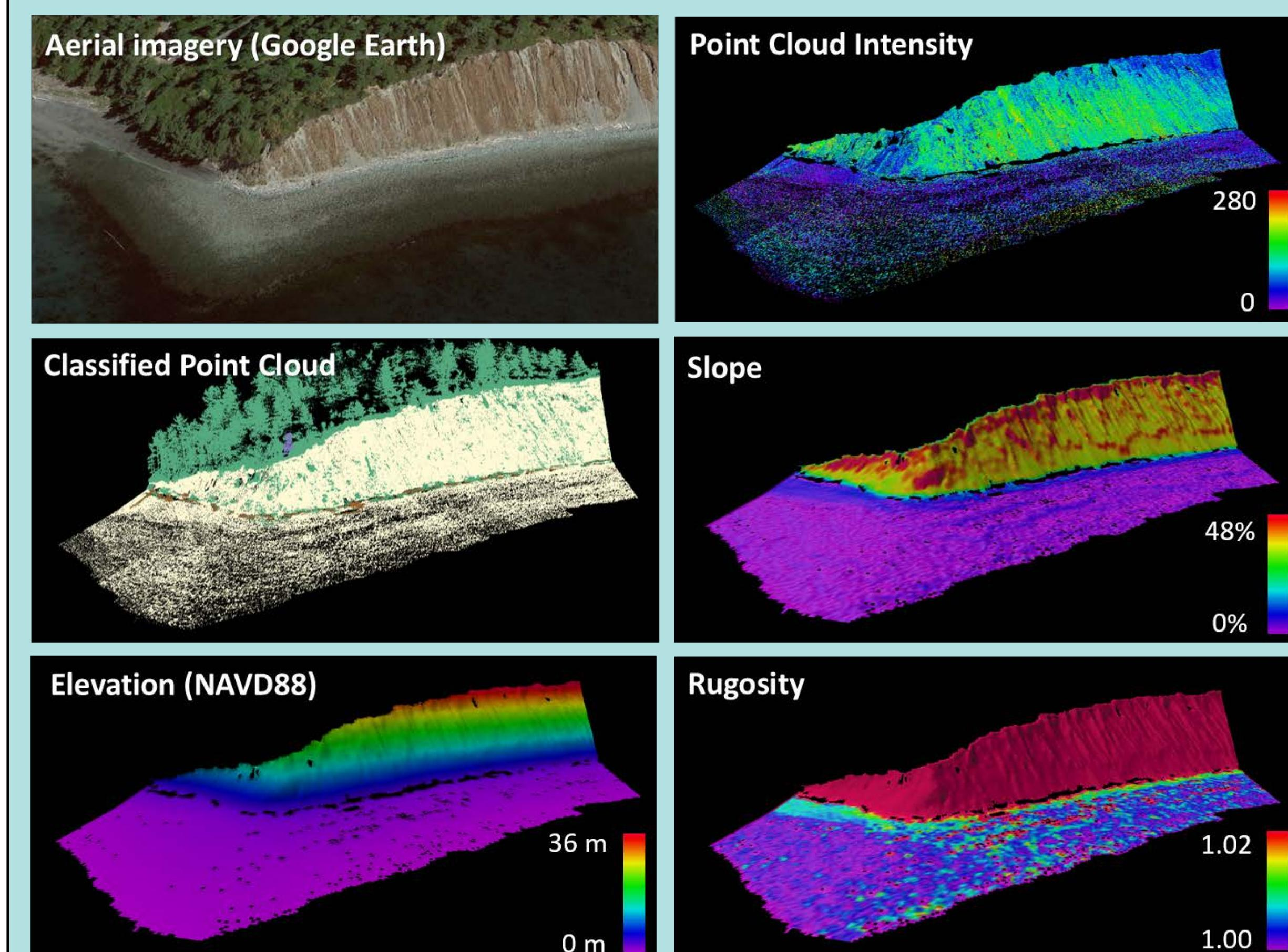
Quantitative measurements determined from lidar point clouds and digital elevation models (DEMs) can be compared to determine natural regional variability and the effects of shoreline modifications on process, structure, and function. Certain features provide metrics to assess nearshore habitat that are crucial for prioritizing ecosystem protection and restoration, and recovery of salmon, orcas, and marine birds.
