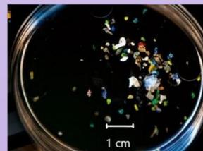
Figure 8: Microplastic fragments in petri dish
