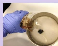
Figure 5: Sieving lithium metatungstate separated sediment
