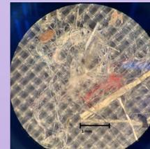
Figure 9: Microplastic fibers in 0.33 mm sieve
