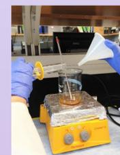
Figure 6: Wet peroxide oxidation
