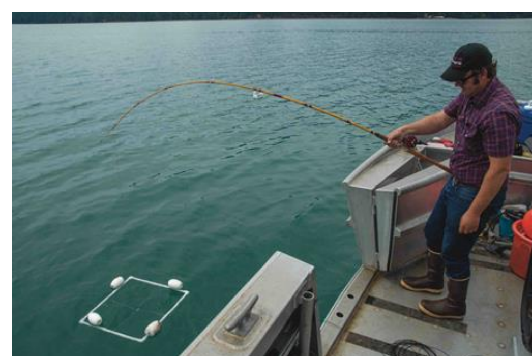
Figure 3. Depth profile sampling of irradiance
