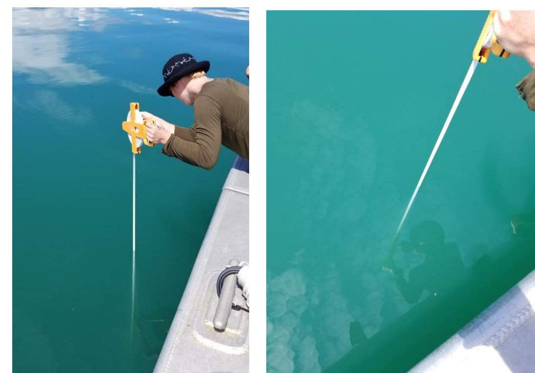
Figure 4. Visibility measured using Secchi disk
