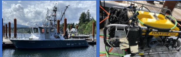
Image 3. The MV Manyberries, our ship platform (left) and the ROV, "Phantom HD2" (right), used for seafloor surveys
