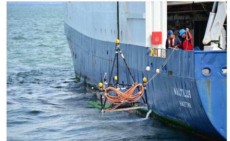
Multi-hydrophone array being deployed in the Strait of Georgia, 2015
