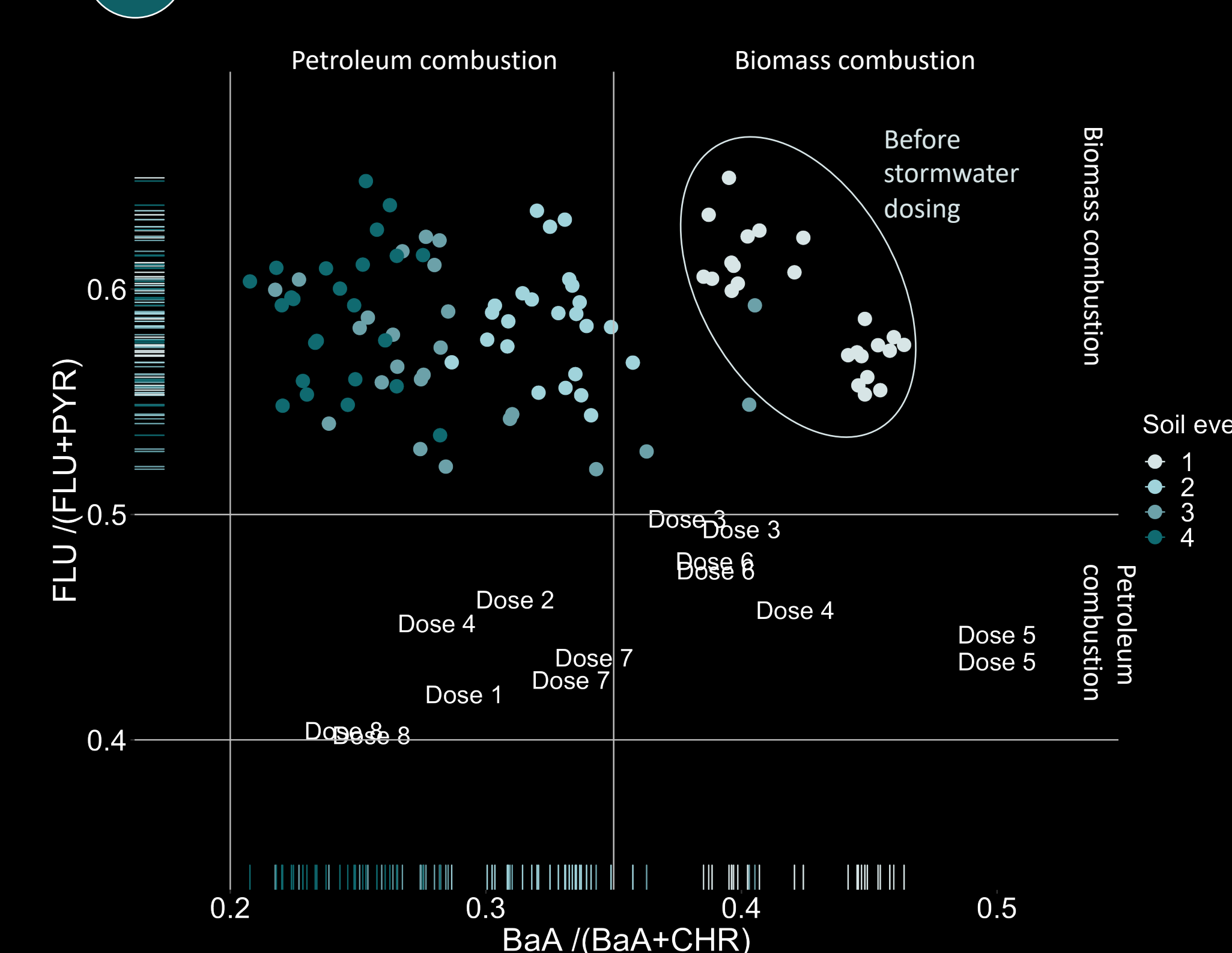
Figure 2. Diagnostic ratios of benzo(a)anthracene/chrysene and fluoranthene and pyrene for soil samples taken across 4 soil sampling events (points) and for influent samples across all dosing events (text). Duplicate influent samples are plotted.
