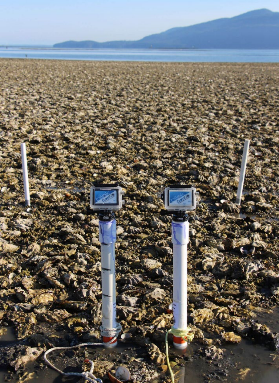
TWO CAMERAS STAND ABOVE A SECTION OF AN OYSTER FARM IN SAMISH BAY, WASHINGTON, AT LOW TIDE. THEY BECOME SUBMERGED AT HIGH TIDE AND COLLECT UNDERWATER VIDEO OF MARINE LIFE INHABITING THE AREA. PHOTO BY NORTHWEST FISHERIES SCIENCE CENTER.
