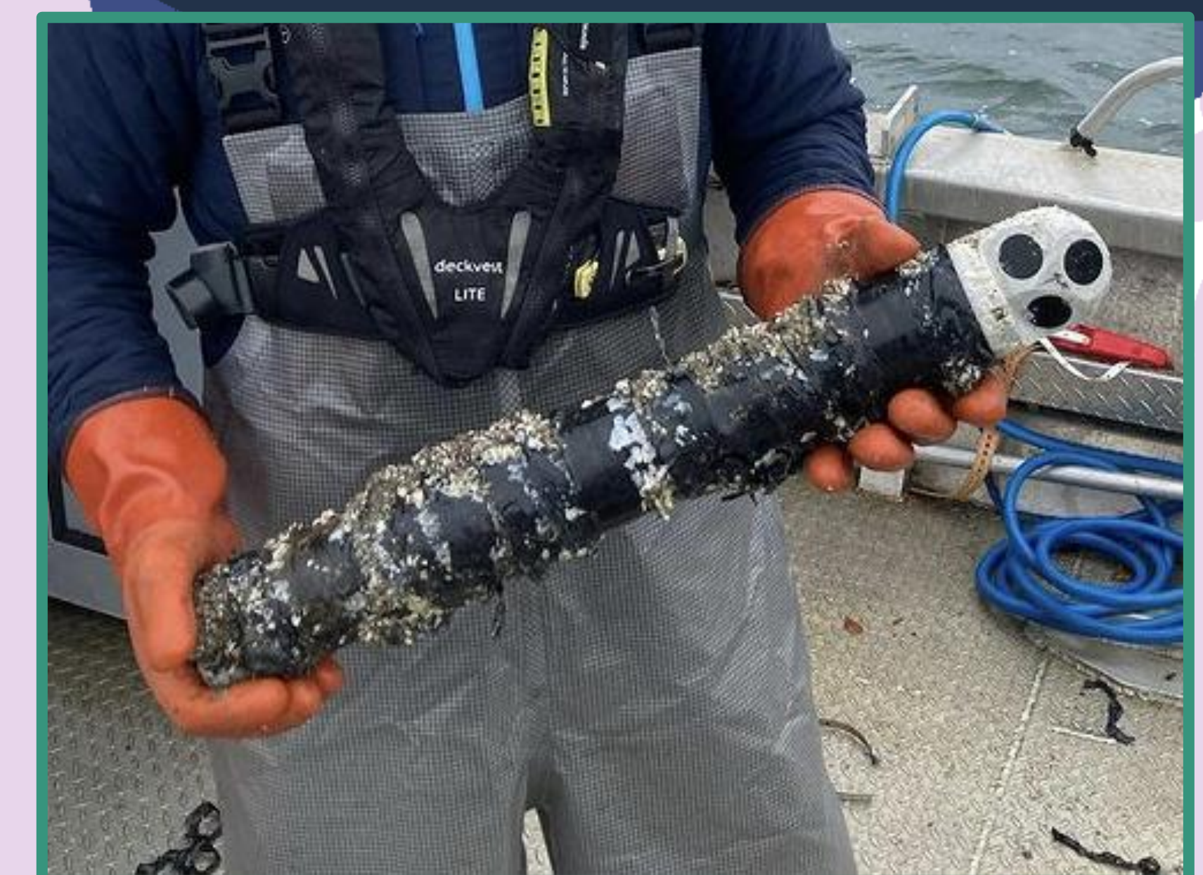
Fig. 1 - Photo of someone holding up the ADCP that was used to collect current velocity data
